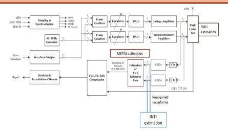
Component 1: Development of reference system for calibrating PMUs
