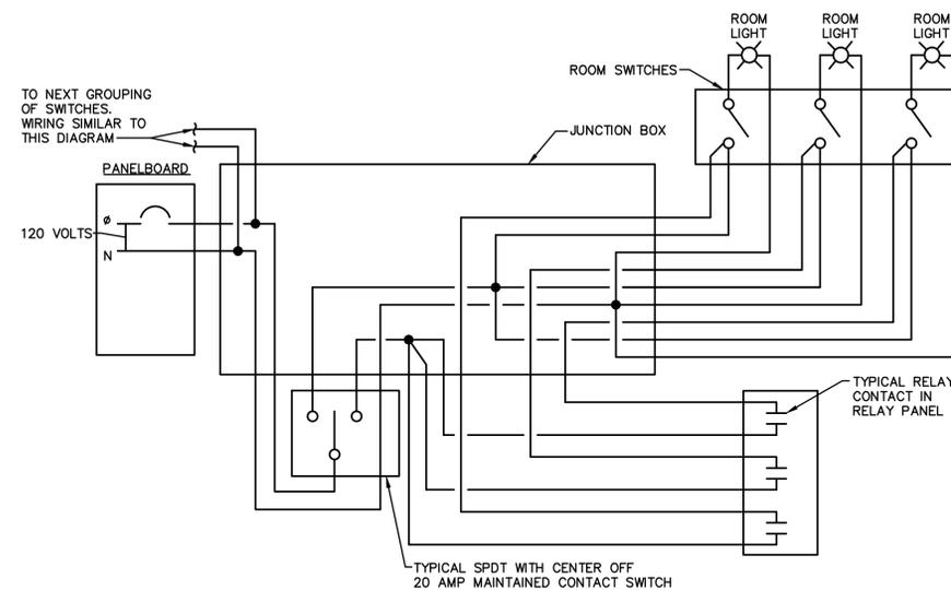
**TYPICAL FUTURE WIRING DIAGRAM FOR ROOM SWITCHES**
