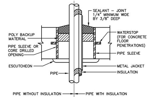
**PIPE SLEEVE THRU FLOOR DETAIL**
