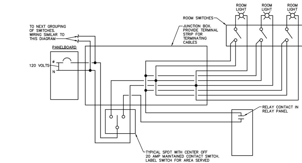
**TYPICAL WIRING DIAGRAM FOR ROOM SWITCHES**
