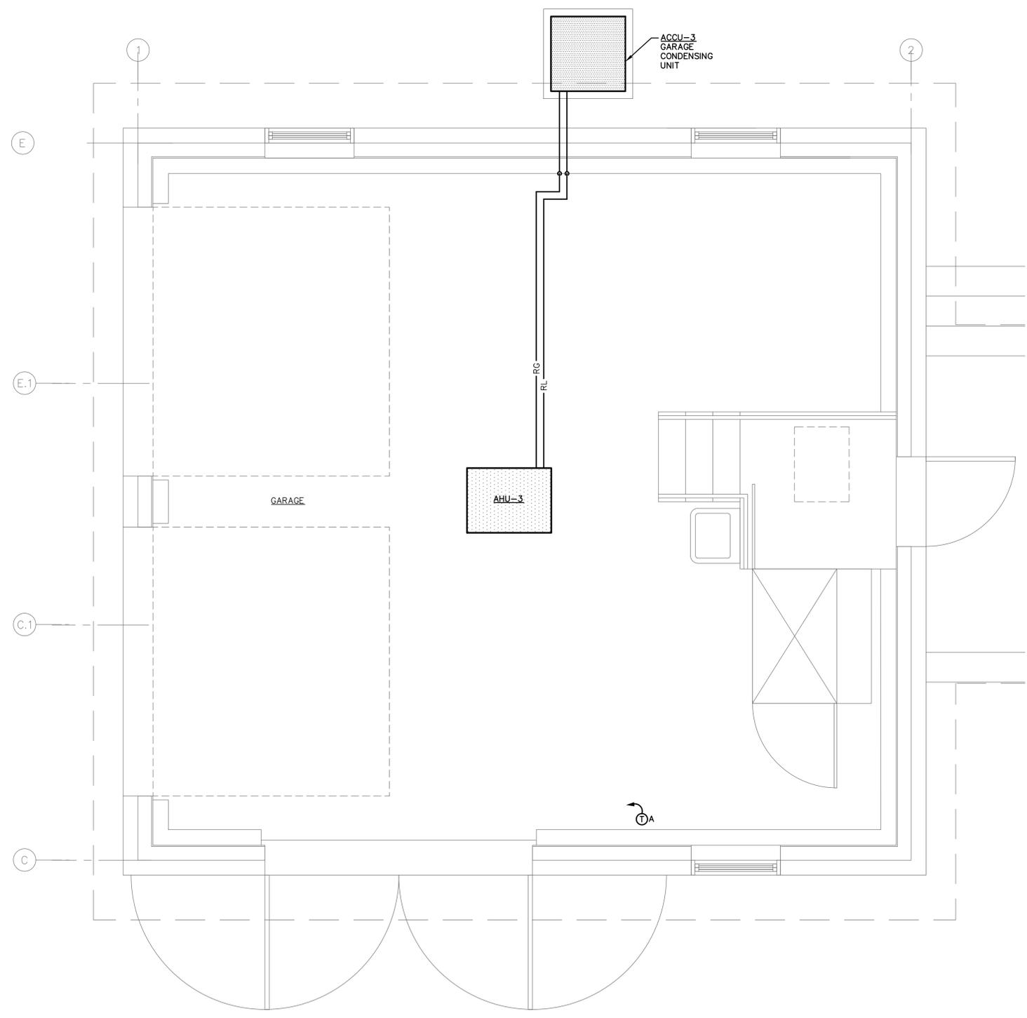
**FIRST FLOOR PLAN GARAGE - HVAC**
