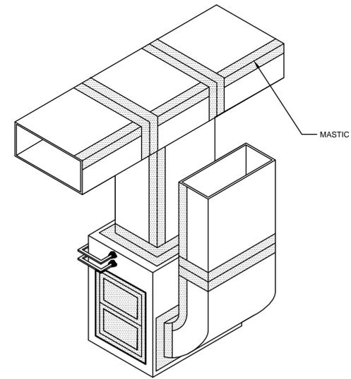
**AIR HANDLER AIR SEALING DETAIL**
