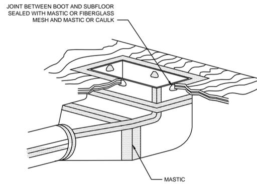
**FLOOR BOOT AIR SEALING DETAIL**
