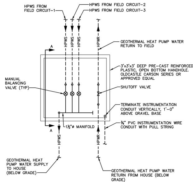
**GEOTHERMAL SYSTEM VALVE HANDHOLE DETAIL**
