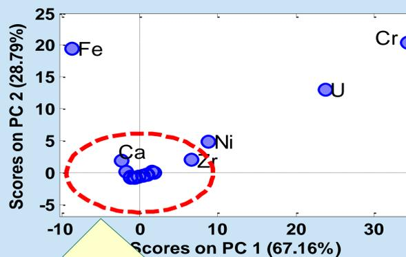
**Figure 1:** PCA results for one sample of SRM 4600. The red ellipse denotes three standard deviations from the center of the PCA model built on the XRF 'stability run' data obtained for this sample. The PCA model suggests that four elements (Cr, Fe, Ni and U) lie outside the ellipse and exhibit detectable "nugget effects" or sample heterogeneity.
