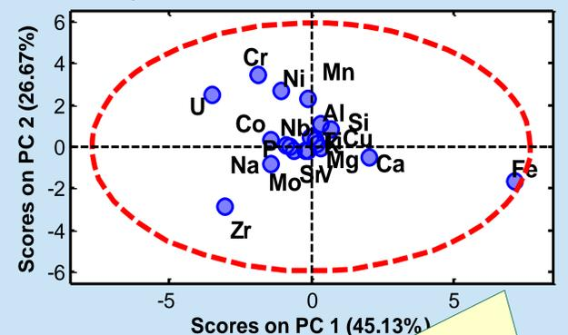
**Figure 2:** PCA results after averaging 250 spectra from SRM 4600. All elements fall within the red confidence ellipse indicating no measureable nugget effects at a sample size of 1 mg.
