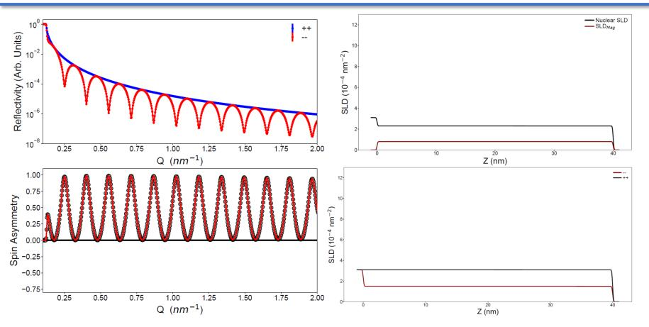
One can sometimes find systems where  $\rho_N^{\text{Substrate}} = \rho_N^{\text{Film}} + \rho_M^{\text{Film}}$  for one of the two spin states. In this case we expect oscillations in one of the spin-states and a R ~ Q<sup>-4</sup> dependence for the other.
