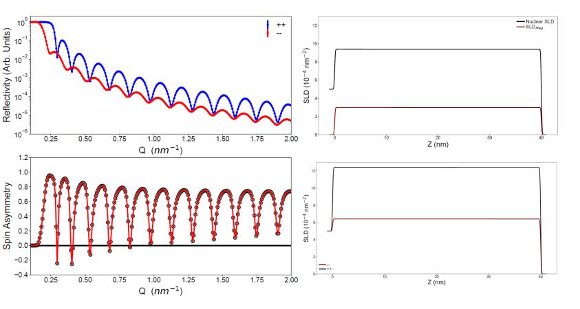
Here we see the simulated reflectivity of a 40 nm thick Ni film on MgO over a Q-range of 2 nm<sup>-1</sup>
