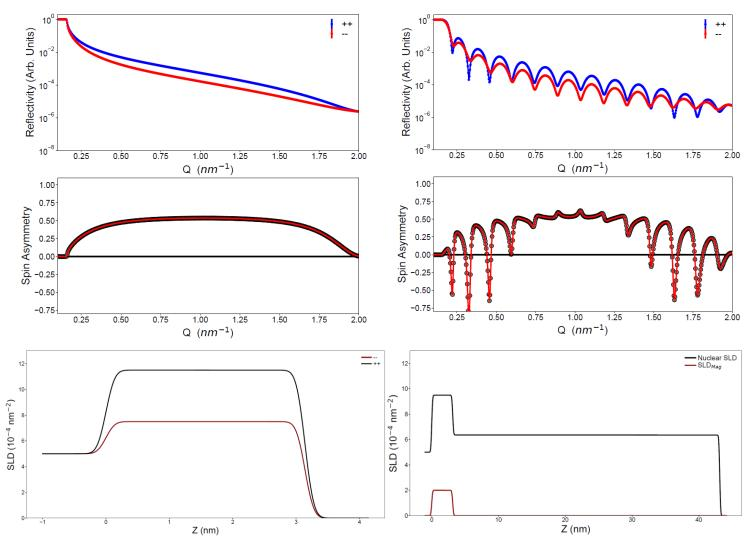
Here we see that the thick capping layer creates high-frequency features in the spin asymmetry, but the envelope function associated with the magnetic layer remains.
