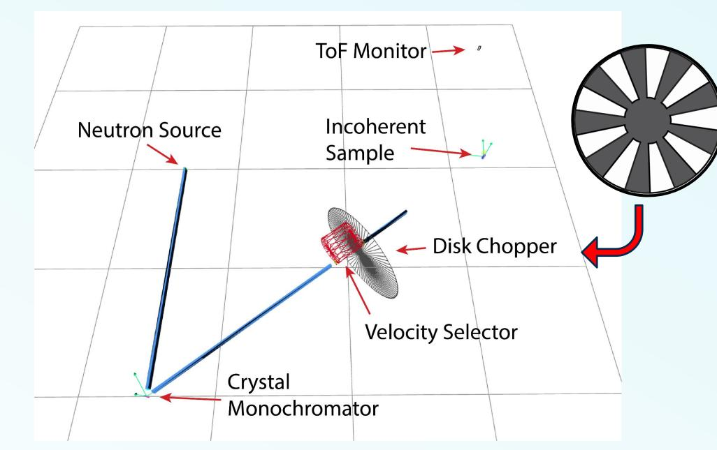
Following scattering, differences in neutron velocities will smear the triangular profile over time. By measuring the Fourier components of this smear, we can obtain the Fourier transform of the dynamic structure factor, S(Q,E).
