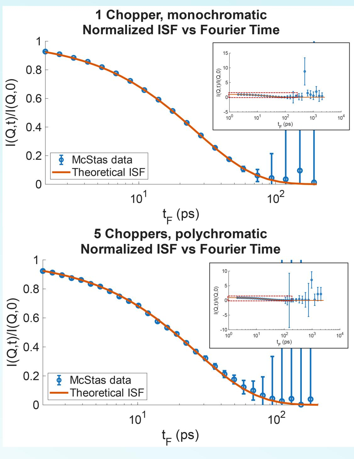
The agreement up to 10<sup>2</sup> ps indicates that both variations of NIMS are realistically appropriate to probe timescales of molecular, atomic, and spin motions of up to 10<sup>2</sup> picoseconds, corresponding to ≈10µeV energy resolution.
