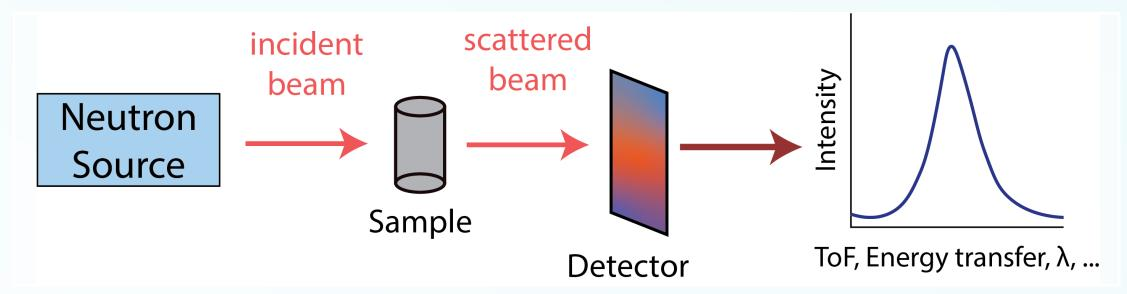
One of the largest limitations of current QENS instruments is the loss of neutron flux from the typically prerequisite pulsation and monochromation of the incident beam.
