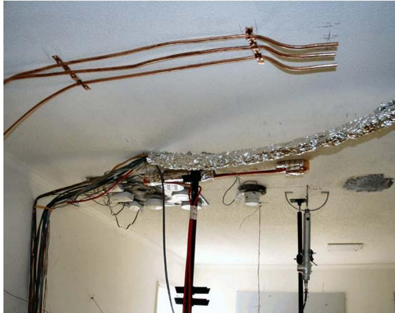
Figure 96. Smoke properties measurement showing collection lines (foreground) and smoke velocity measurement (background)
