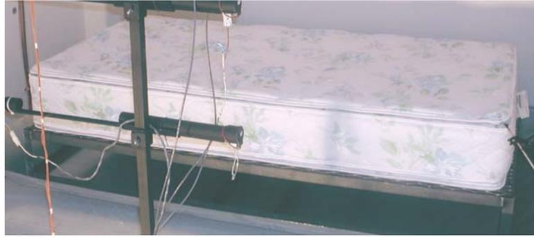
Figure 81. Mattress used for smoldering and flaming experiments
