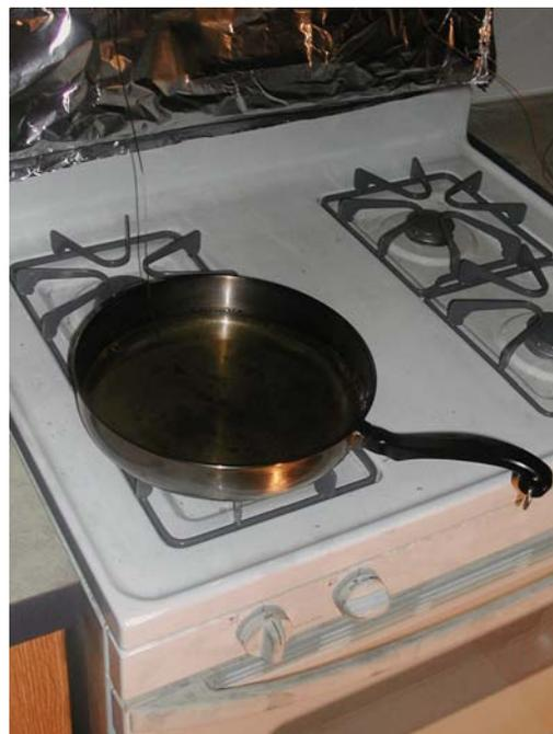
Figure 86. Heating ignition source with cooking oil
