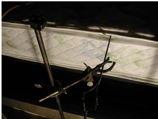
Figure 85. Rod used for smoldering ignitions
