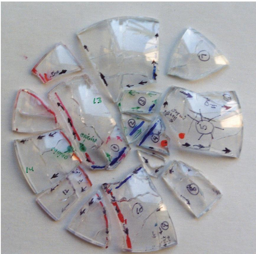
Fracture of a sapphire missile nose cone. Credit: NIST
