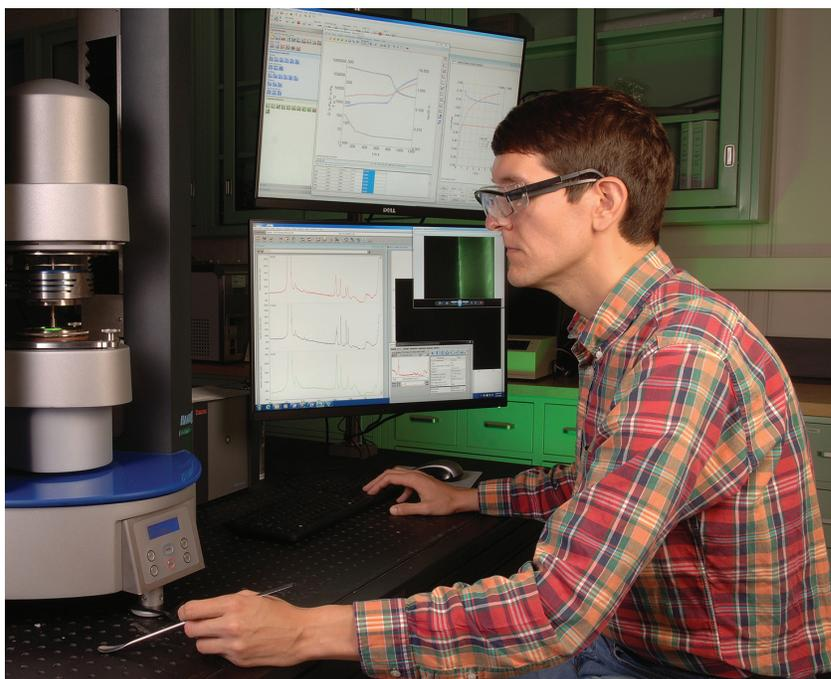
NIST’s Anthony Kotula using the new rheo-Raman microscope, a three-in-one instrument that enables researchers to measure the flow properties of a material along with its microscopic structure and composition. Credit: Denease Anderson/NIST
