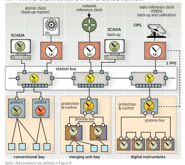
IEEE 802.1D bridge functionality does not apply to 1588. So even ports blocked by the Rapid Spanning Tree Protocol send (modified) Sync messages.
