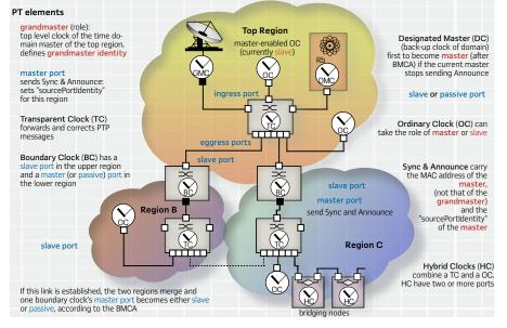
Therefore, IEC 62439-3 Annex A modifies the 1588 principle exclusively for PTP messages. A slave treats the master clock seen on LAN A and LAN B as two different clocks and applies a Best Master Clock algorithm to select its master.
