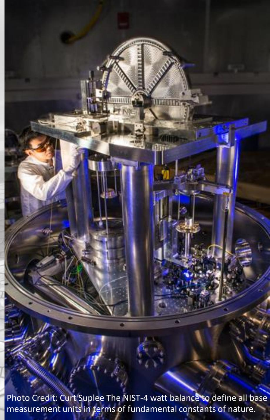
Photo Credit: Curt Suplee The NIST-4 watt balance to define all base measurement units in terms of fundamental constants of nature.
