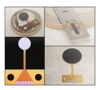
Clockwise from upper left: bolometer for optical fiber power measurement operates at 4K, bolometer for space-based measurement of solar spectral irradiance, operates at room temperature; bolometer for continuous wave, visible/near infrared laser power measurement, operates at room temperature; bolometer for fast far infrared power calibration, operates at 4K.
