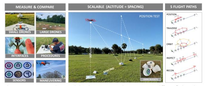
The Open Test Lane uses designated altitudes, positions, and orientations in 5 different flight paths to evaluate Basic Maneuvering and Payload Functionality. All flights are conducted in open environments with no obstacles.
