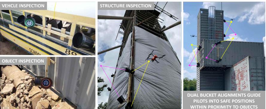
The Obstructed Test Lanes and related scenarios enable remote pilots to fly safe and repeatable flight paths to inspect objects from close proximity. There are 5 different tests that guide remote pilots through various standoff positions, orientations, and perches at 2-3 m (6-10 ft) from objects. These tests can be performed outdoors or indoors to control lighting, weather, and access to GPS.
