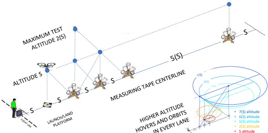
**OMNI STAND SPACING = S    MAX TEST ALTITUDE = 2(S)    LANE LENGTH = 10(S)**
