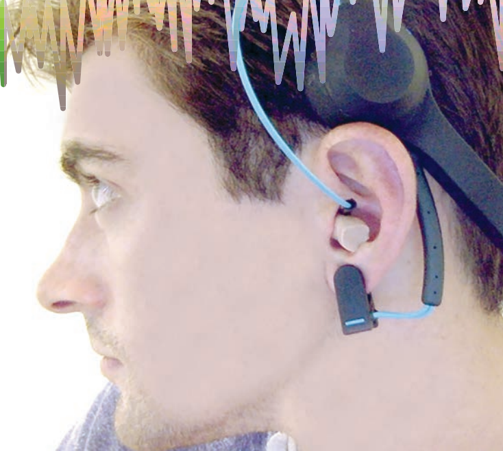
A UC Berkeley engineering team uses these earbuds to record brainwaves. They created the earbuds themselves using a 3D printer.
