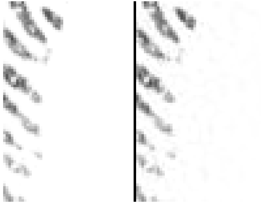
Figure 71: Artifacts at the boundary of a fingerprint resulting from WSQ compression (factor 8).
