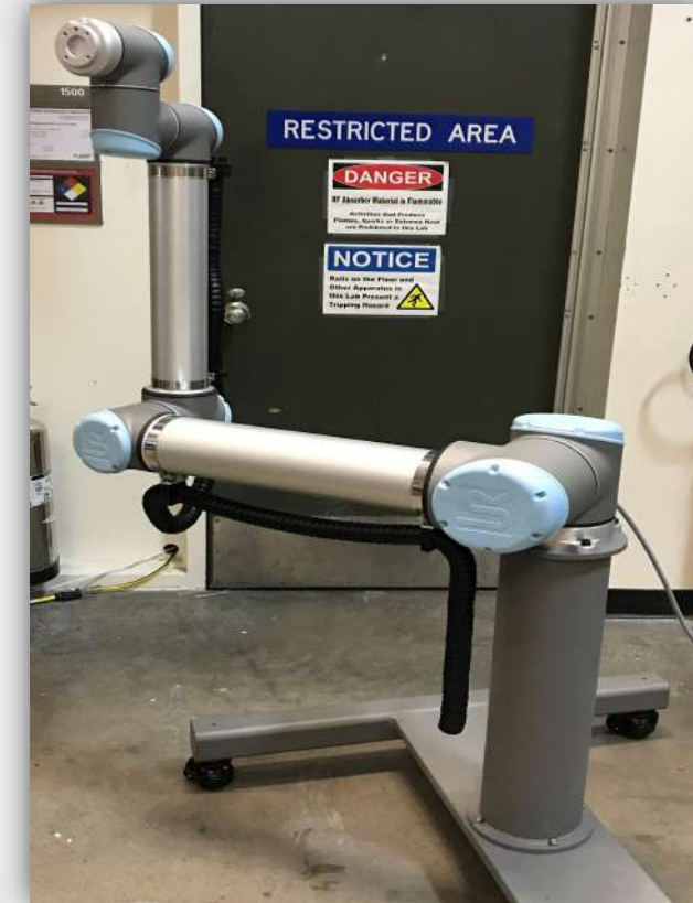
Robotic arm with 6 degrees of freedom
