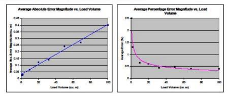
Absolute error magnitude tends to increase roughly proportionally to measured volume. Percentage error magnitude tends to a relatively constant (or slightly improving) value with increasing volume.
