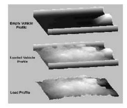
The LVS measures the load <u>as it sits in the truck at the time of measurement</u>. The measured volume is the "loose" volume generated by the surface contour and it makes no assumptions about product density or changes in volume over time.
