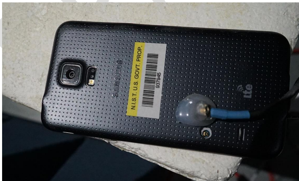
Figure A-4. The UE used in Phase I measurements, shown with the hardline attached to one of the RF ports.
