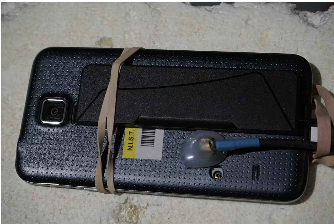
Figure A-6. The Phase I test UE is shown with the passive coupler banded to it.
