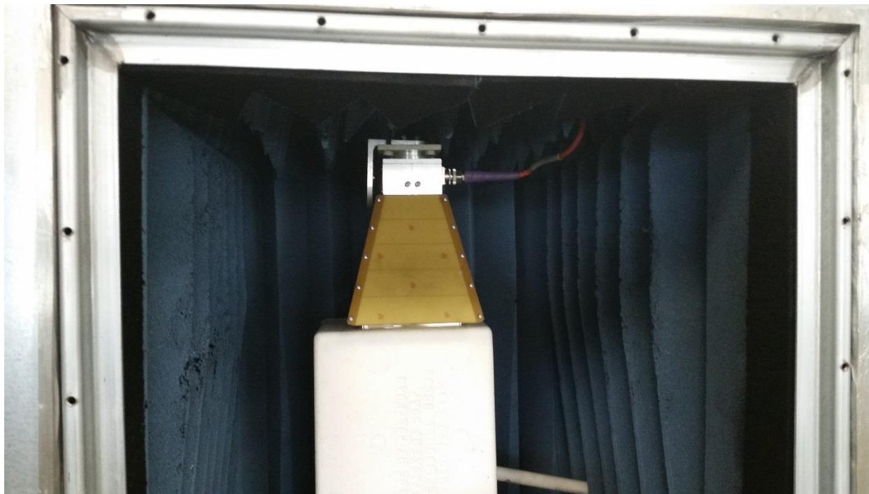
Figure A-5. The UE placed inside the small anechoic chamber during the coupled/radiated testing. The UE is placed on top of foam blocks, and appears as a silver line immediately underneath the horn antenna.
