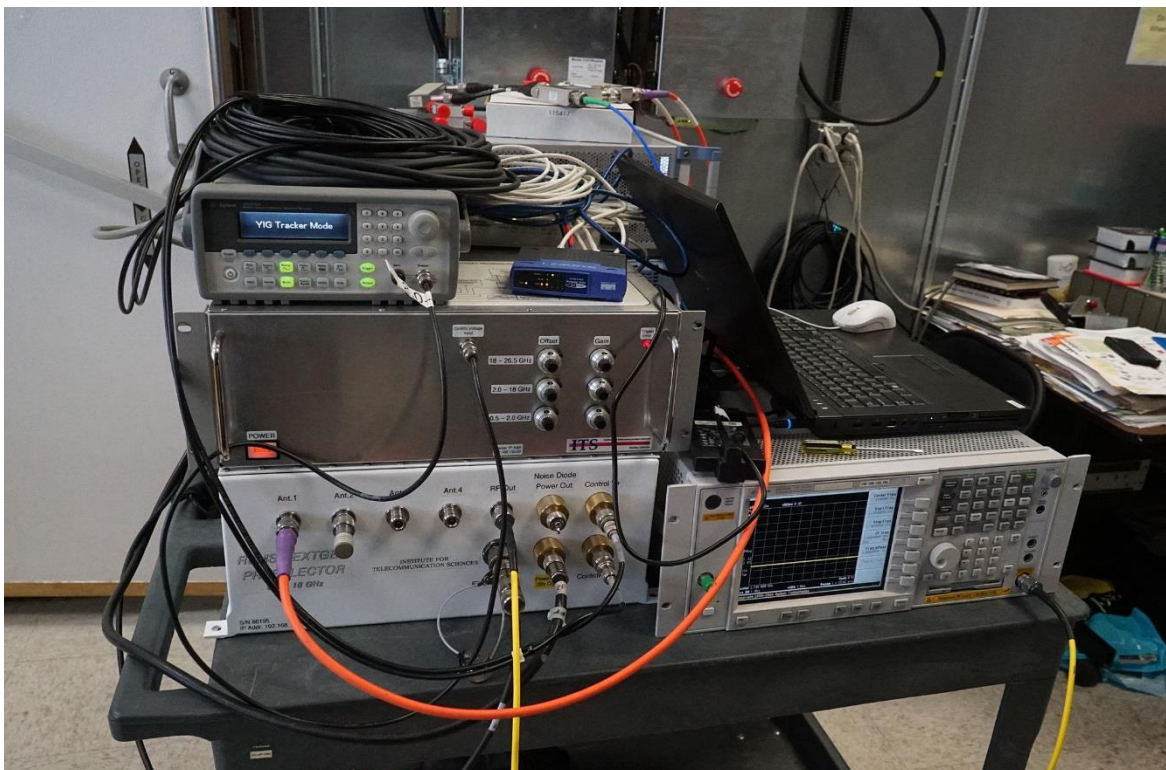
Figure A-3. The spectrum analyzer (bottom right), acquisition laptop (on top of the spectrum analyzer), and RF preselector (3 box stack) used for both the UE and eNodeB measurements.
