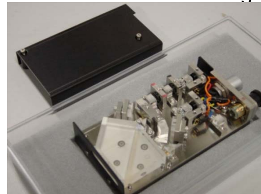
Interferometer optics with double-pass, homodyne detection
