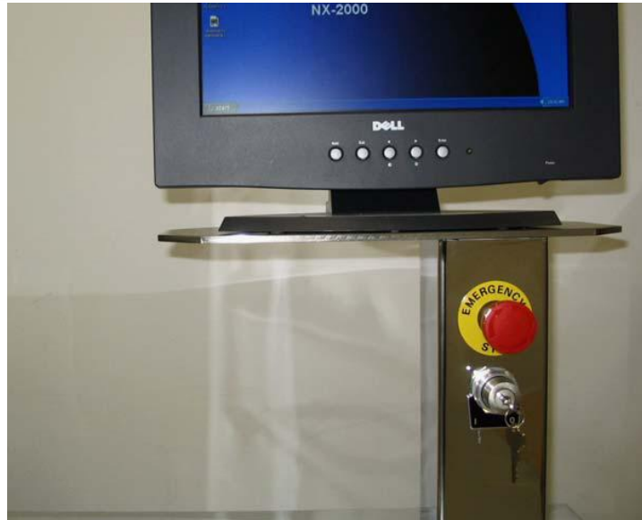
Emergency stop and control key of NX-2000 nanoimprinter
