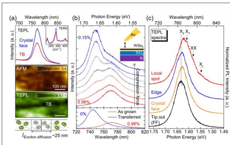
**Fig. 1.** (a) TEPL spectra and image of the as-grown ML WSe<sub>2</sub> at crystal face and twin boundary regions. (b) Evolution of TEPL spectra with increasing compressive force by the tip, giving rise to a release of the tensile strain of the crystal.
