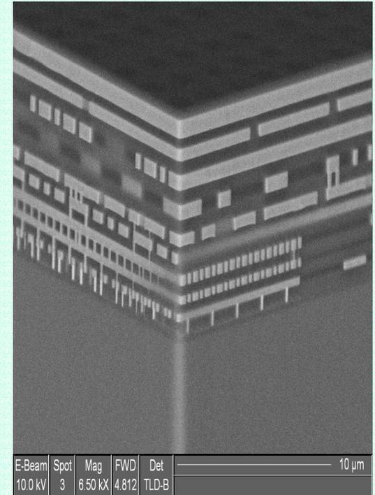
Half of the Structure and Cost of an IC is Interconnects
