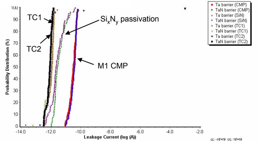
Leakage current probability plot for 4 sequential etest steps.
