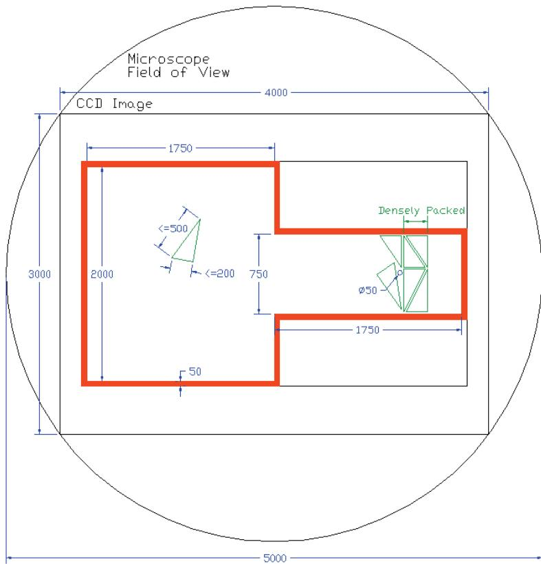
**Figure 2: Arena Dimensions for the Microassembly event**
