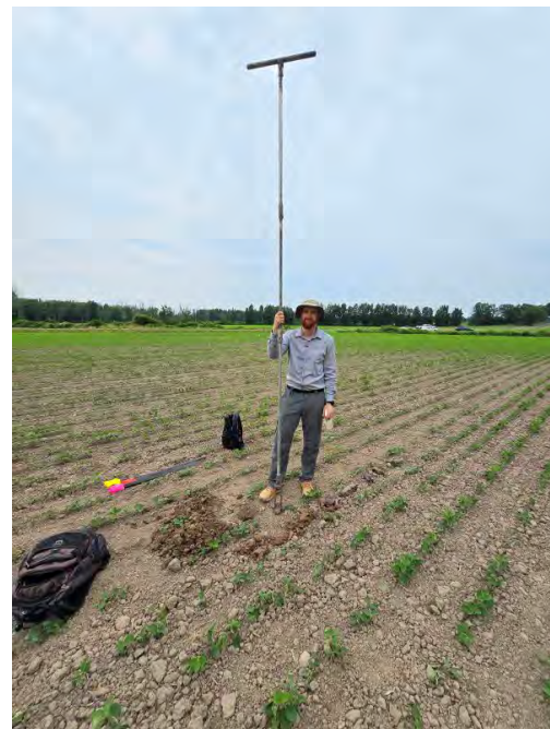
Reed 1 (digging a deep test hole using a 10.5-foot-long soil auger)
