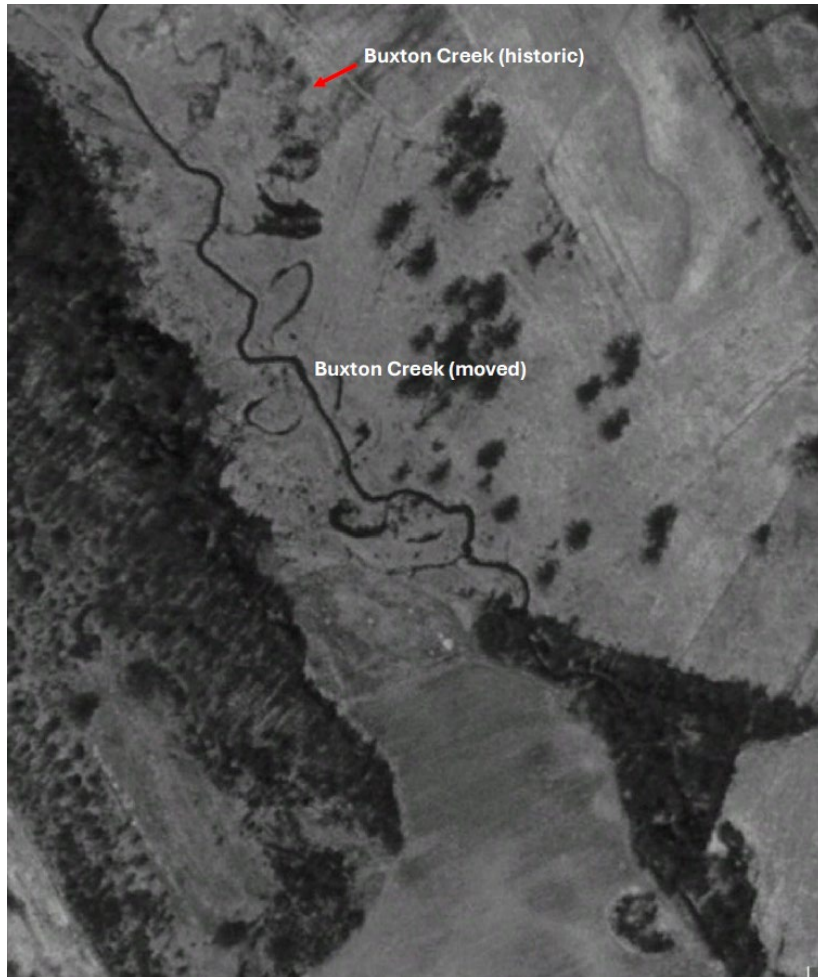
Figure 8-2a. Buxton Creek North of Bell Road
