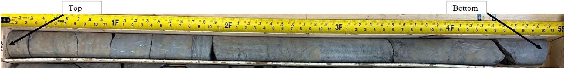
Photograph 1 Boring: B-227 Run 1 Depth 24.0' - 29.0' See Photograph Nos. 2 and 3 for detailed views.
