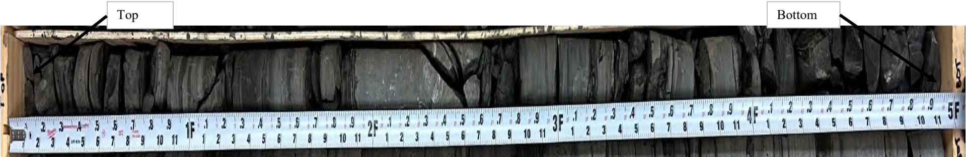
Photograph 46 Boring B-426 Run 1 Depth 22.5' - 27.5' See Photographs Nos. 47 and 48 for detailed views.
