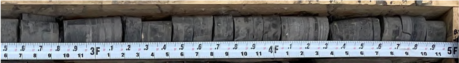
Photograph 12 B-30 Run 1 Bottom Depth 21.5'-24.0'
