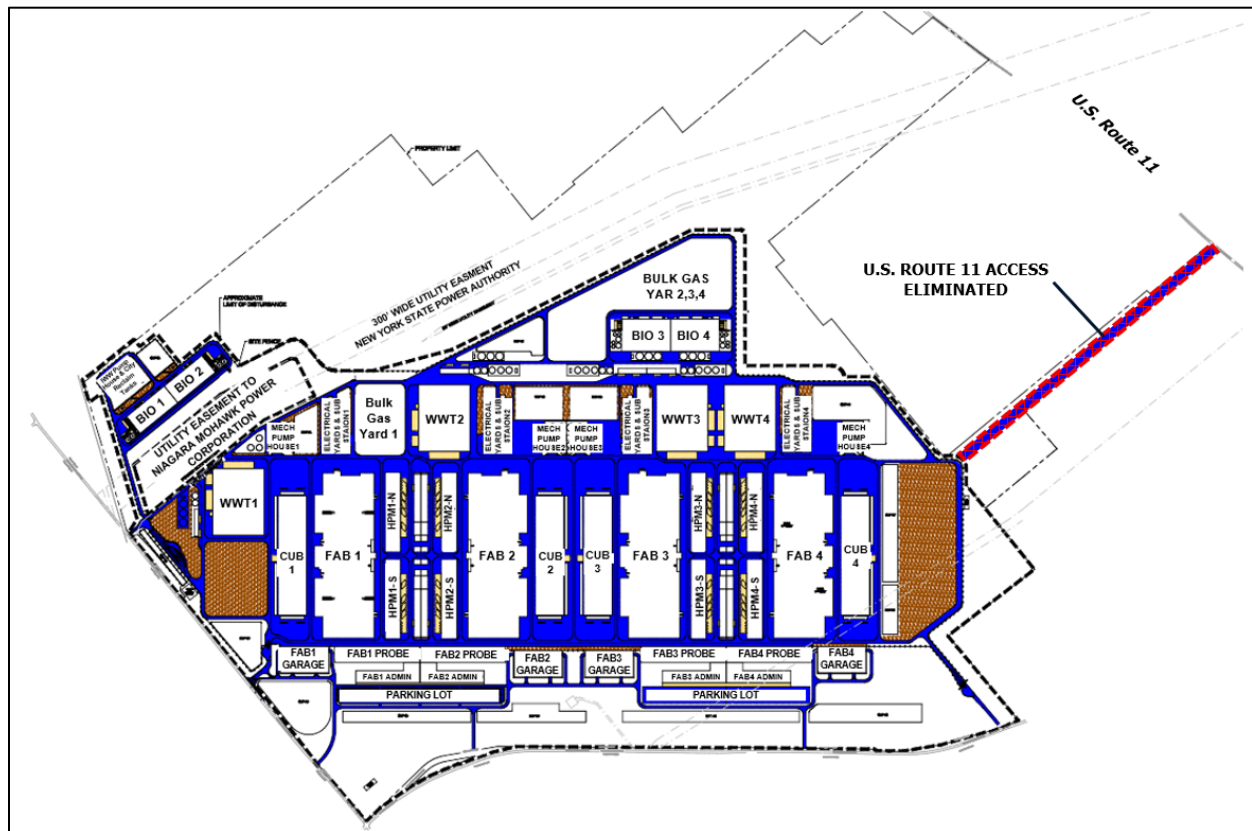
Figure 2.2-2 U.S. Route 11 Access Elimination Layout
