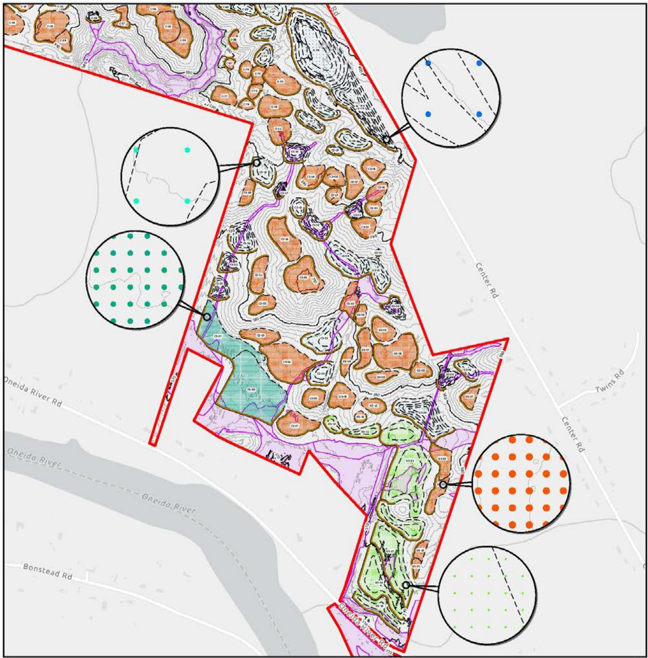
Figure 5-5. Wetland Grading Plan- Southeast
