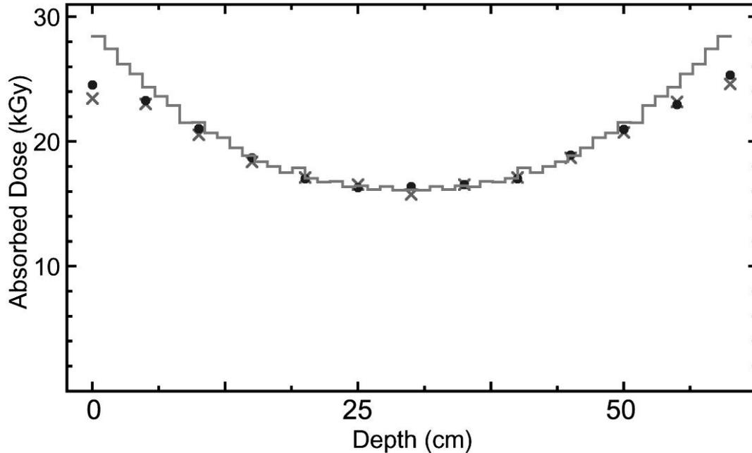
**Figure 5. Depth-dose distribution through totes filled with paper: Monte Carlo calculation (-); alanine dosimetry in the middle tote (x) and end tote (•).**
