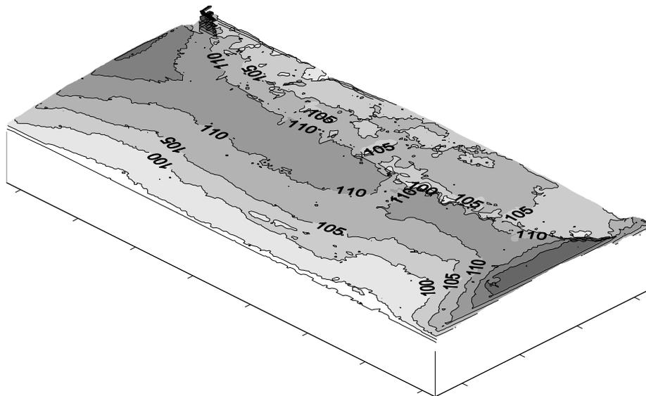
**Figure 2. Radiochromic-film map of dose distribution within the plane of an envelope (doses in kGy). The dark mark in the upper corner of the image is for identification.**
