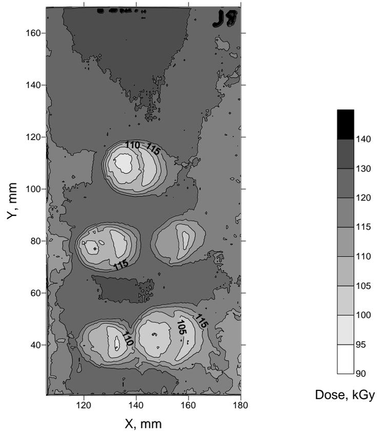
**Figure 1. Radiochromic-film dose map mounted against coins in an envelope. The dark marks at the top of the image are for identification.**
