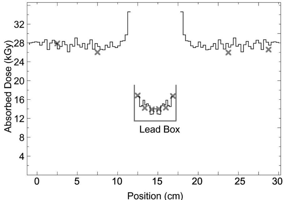
Figure 4. Depth-dose distribution through a lead box: Monte Carlo calculation (—); alanine dosimetry (x).
