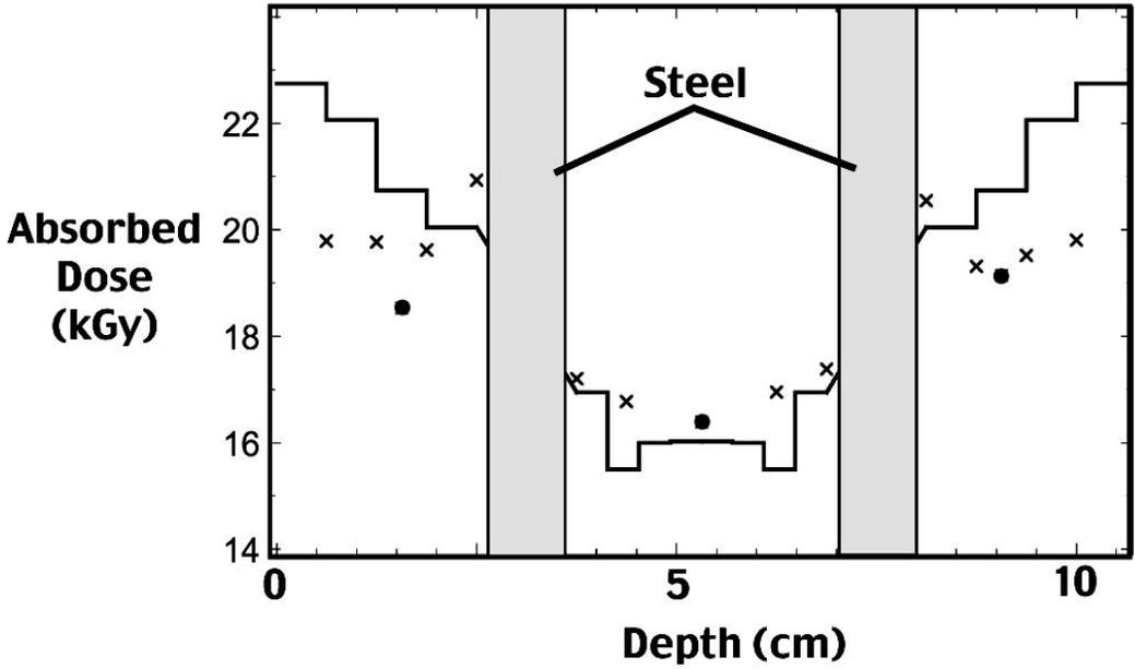
Figure 3. Depth-dose distribution through steel plates: Monte Carlo calculation (—); alanine film dosimetry (x); and alanine pellet dosimetry (•).
