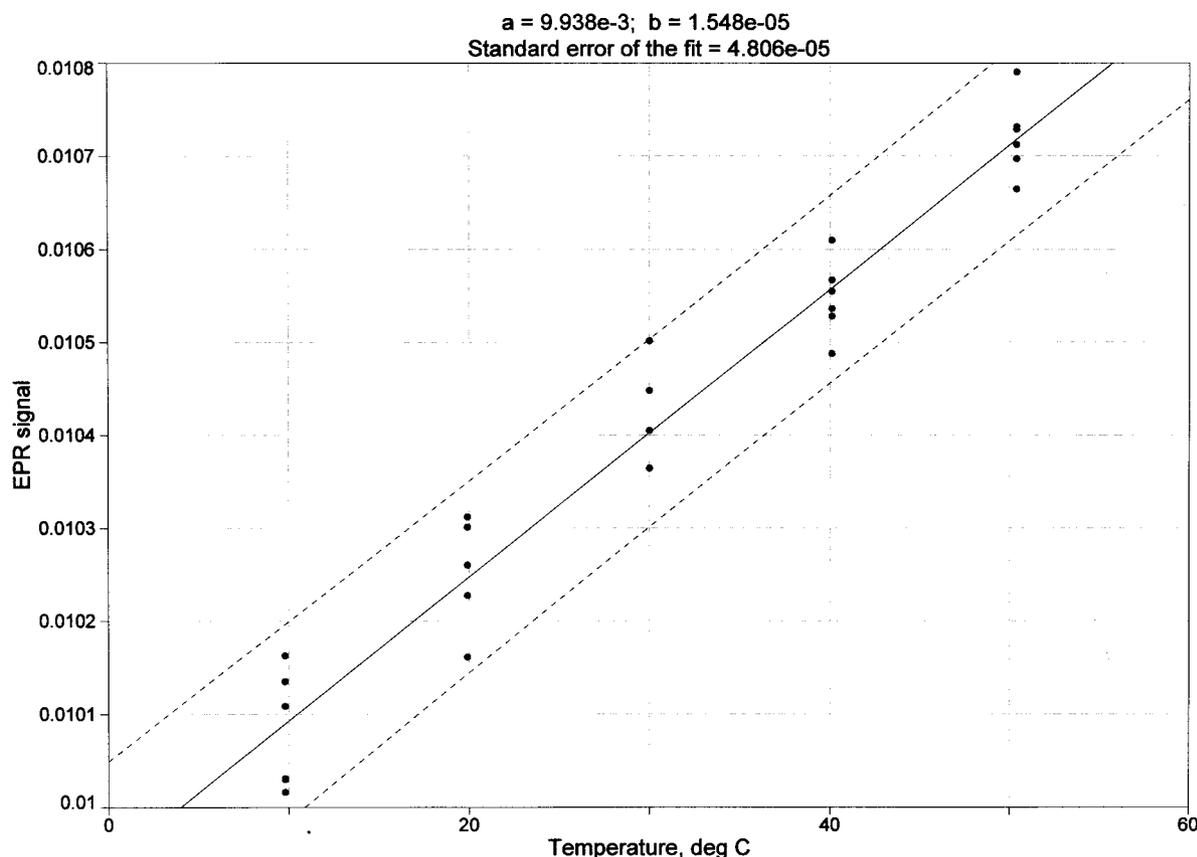
Fig. 2. A typical plot of the alanine dosimeter response on irradiation temperature using Bruker dosimeters (dose 13 kGy). Some of the closely positioned points are not resolved. The dotted lines show the prediction band; no outliers occur in this experiment.
