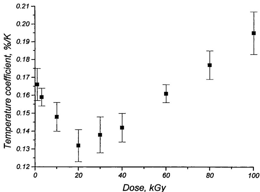
Fig. 6. Dose dependence of the temperature coefficient for NIST dosimeters. The error bars show uncertainties calculated as described in Section 2.4.
