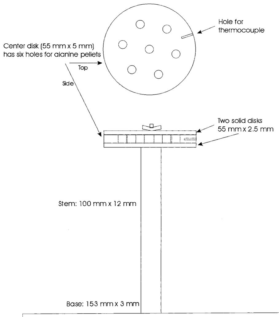
Fig. 1. Aluminum holder used for dosimeter irradiation at controlled temperatures.
