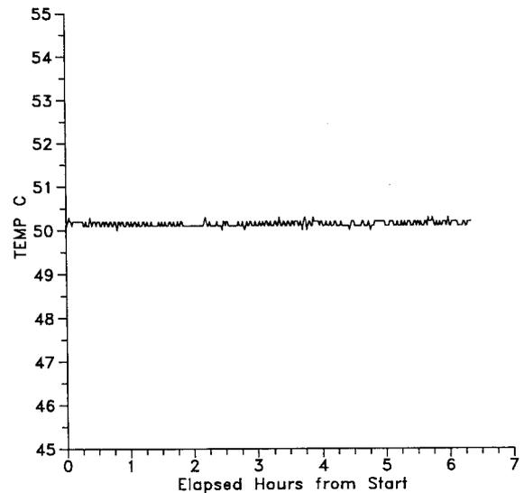
Fig. 4. Variations in the temperature of the thermostatted aluminum during the 1.25-h pre-irradiation period and 5-h irradiation at a dose rate of 9.5 kGy/h.
