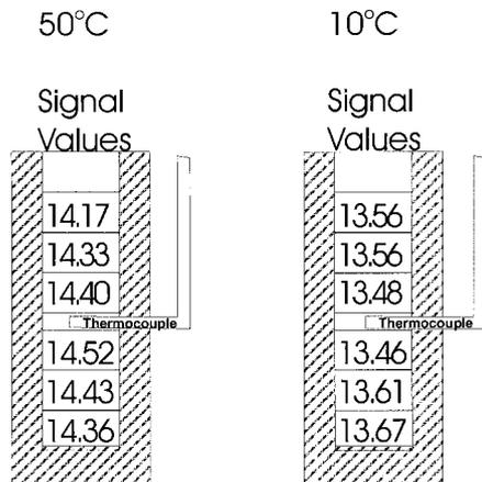
Fig. 3. Dependence of the EPR responses of alanine dosimeters on their position in a polystyrene vial with a thermocouple inserted in the vial center. The vials with the dosimeters were kept at the specified temperatures for 45 min, the subsequent irradiations to 10 kGy took about 1 h.
