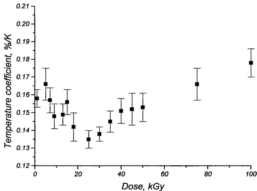
Fig. 5. Dose dependence of the temperature coefficient for Bruker dosimeters (Batch No. 3). The error bars show uncertainties calculated as described in Section 2.4.
