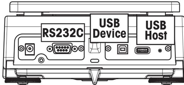
Interfaces and possible connectivity of peripheral devices:
