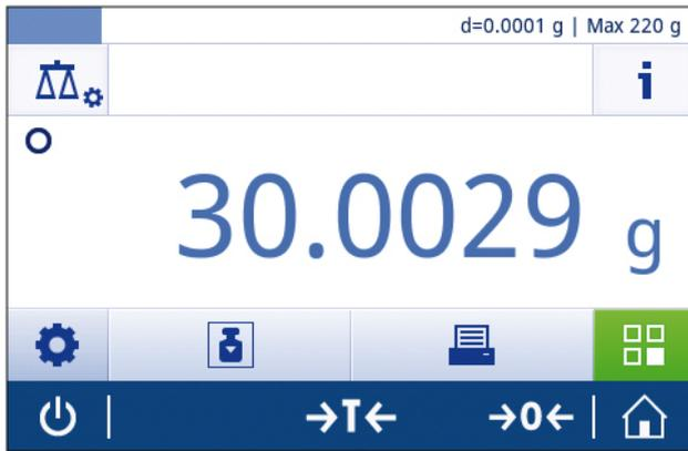
⇒ After a short period of time, the weighing pan is stable. The instability symbol
