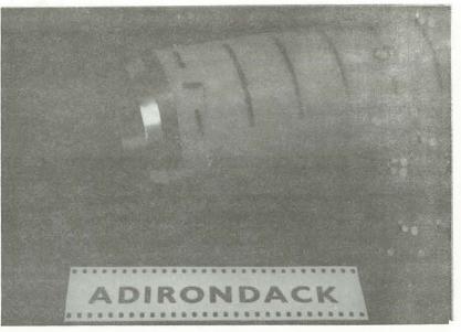
FIGURE 135 The Adirondack sampler has been used widely in shallower snowpacks throughout eastern United States and Canada.
