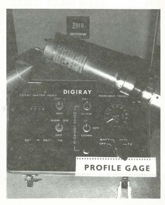
FIGURE 158 The Digiray Portable Profile
