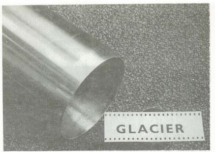
FIGURE 134 The Glacier sampler was used to determine "true" snow water equivalent in all tests made by the Metrication Commuttee.
