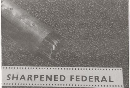
FIGURE 147 The sharpened Federal cutter, is a standard Federal cutter with teeth sharpened to the inside.
