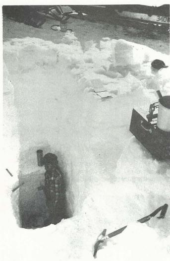
FIGURE 129 Incremental depths are sampled with the Glacier sampler to the ground surface.
