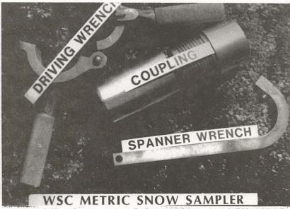
FIGURE 162 The recommended couplings for connecting tube sections, driving wrench, and spanner wrench, for the WSC metric snow sampler.
