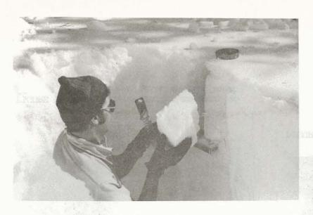
FIGURE 125 A metal plate is placed in the sidewall of the snowpit as a stop for the Glacier sampler.
