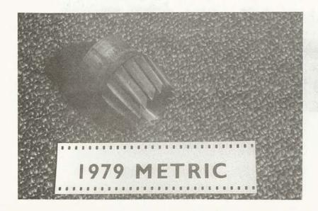
FIGURE 155 The 1979 WSC 10 metric cutter was an evolution of the 1978 long and short metric cutters and had sloping teeth with narrow lands.
