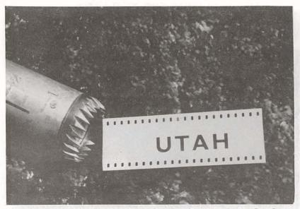
FIGURE 145 The Utah cutter was a 32-tooth early day sampler used with steel snowtubes. This equipment was superseded with the standard Federal sampler.
