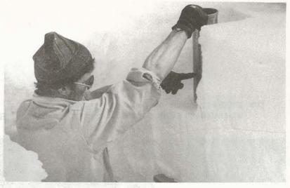
FIGURE 126 The snowpack is sampled in increments of about 35 to 38 cm to determine the snow water equivalent of the entire snow profile.
