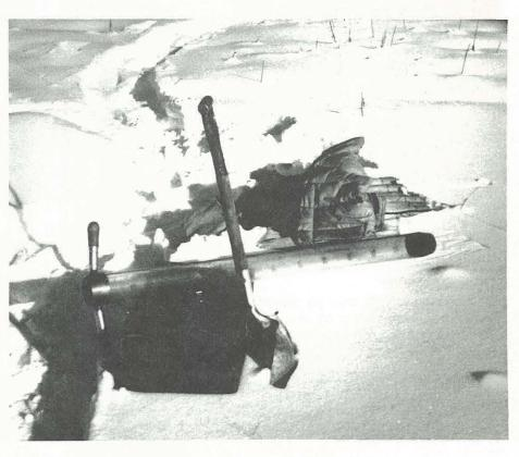
FIGURE 130 Large-diameter samples were obtained in snowpits at same time as small-diameter and Glacier samples.
