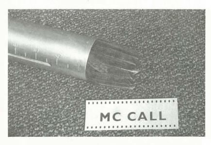
FIGURE 151 The McCall cutter was developed for use in deep dense snowpacks and was used on smooth thick wall tubing with inner couplings.
