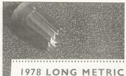
FIGURE 154 The 1978 long metric cutter had the same area as the 1978 short metric but the cutter was similar to the Bowman and McCall type cutters.
