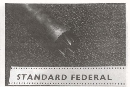
FIGURE 146 The standard Federal cutter is widely used for snow sampling throughout the world.
