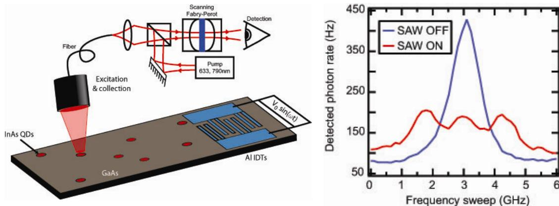
Figure 3.2: **Left:** Schematic diagram of apparatus used to "shake" a self-assembled quantum dot and resolve the fluorescence. **Right:** Fluorescence spectrum of quantum dot (blue curve) acquires resolved sidebands (red curve) when "shaken" by surface acoustic wave.
