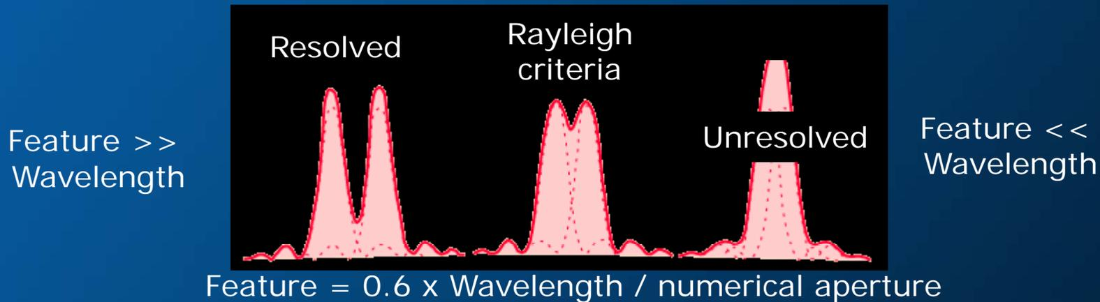
In the limit, microscope objectives with 0.95 N.A. are available and, provided very small fields ( $200\mu \times 200\mu$ ) are adequate, linewidths  $< 0.4\mu$  should be achievable under carefully controlled laboratory conditions, and in very thin resist layers.
