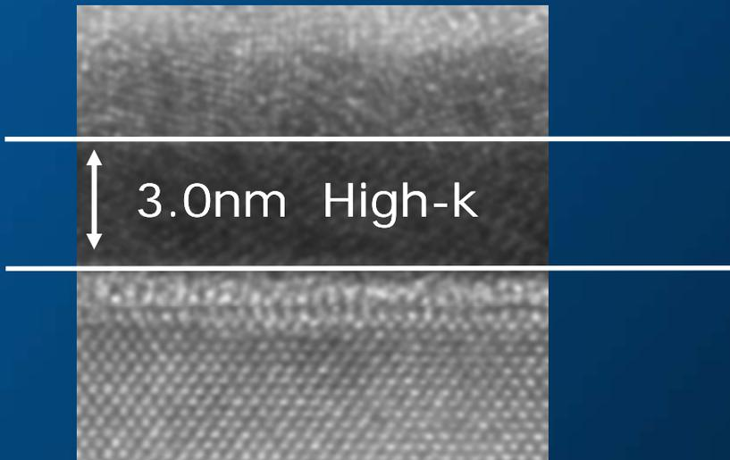
45 nm HK+MG provides >25x gate leakage reduction
