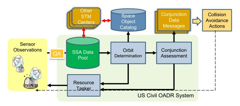
Collision avoidance via STM essential to prevent debris-producing collisions
