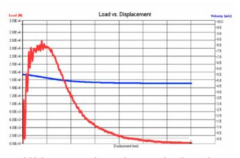
and an energy of 18 J  $\pm$  0.1 J. For low- and high-energy specimens, the uncertainty in maximum force is equivalent or better than the uncertainty in absorbed energy.
