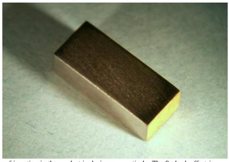
mechanisms for power generation and solid-state refrigeration in thermoelectric devices, respectively. The Seebeck effect is demonstrated by the proportional electric potential that develops across a conductor when placed in an applied temperature difference. The value of this ratio is termed the Seebeck coefficient,  $S = \Delta V/\Delta T$ .
