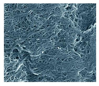
Scanning electron microscope image of a typical sample of the NIST single-wall carbon nanotube soot Standard Reference Material. The nanotubes tend to stick together and form smaller and larger bundles. Some of the impurities also are visible. The image shows an area just over a micrometer wide. (Color added for clarity.) Credit: Vladar, NIST
