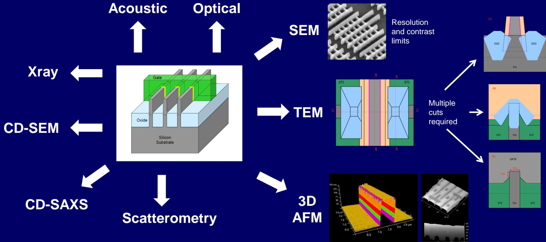
New capabilities to enable critical 3D measurements
