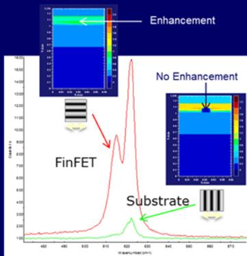
Geometrical FinFET-induced field enhancement enables transistor level measurements
