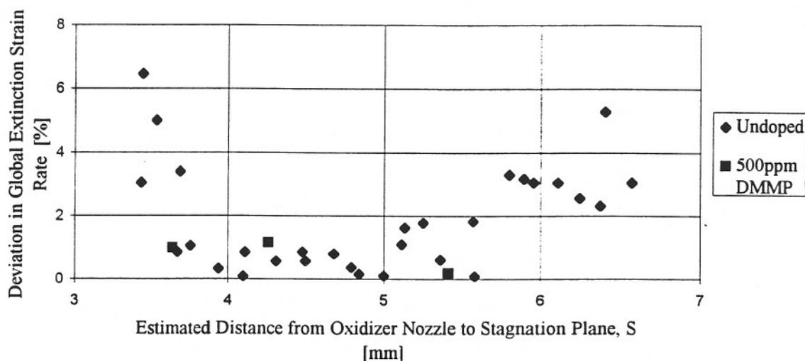
Figure 2. Percent deviation of global extinction strain rate from its mean value in acceptable region. The acceptable region, where deviations are less than 2%, falls where  $S$  is between approximately 3.75 and 5.75 mm.
