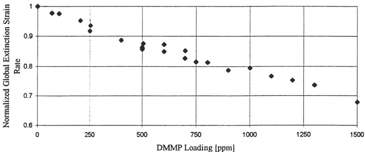
Figure 3. Global extinction strain rate for methane-air non-premixed flames doped with DMMP on oxidizer side. Data normalized to undoped strain of  $431 \text{ s}^{-1}$ .
