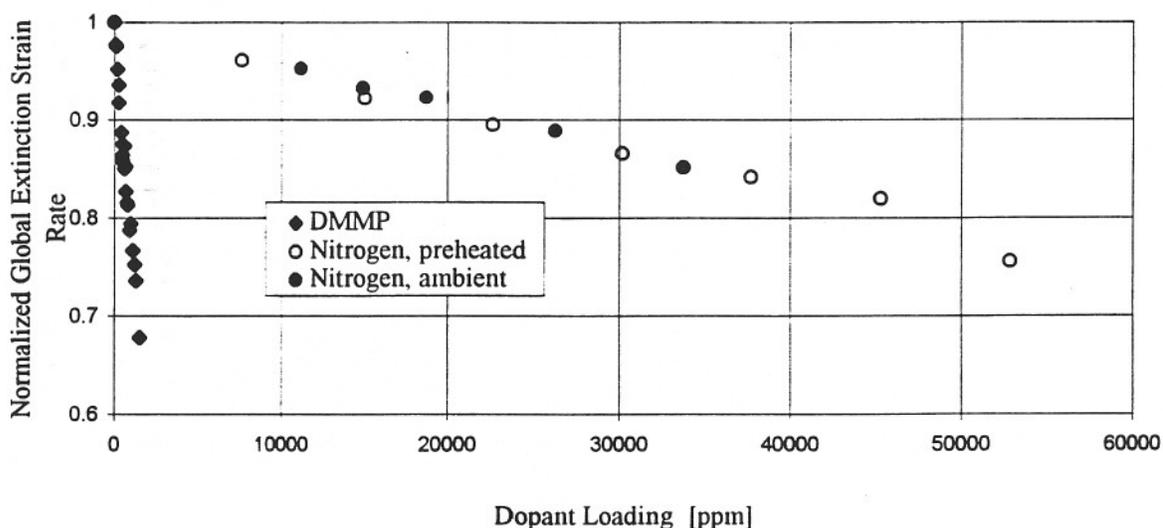
Figure 4. Global extinction strain rates of inhibited methane-air, non-premixed flames doped on oxidizer side. Data normalized to undoped strain of  $431 \text{ s}^{-1}$  for DMMP,  $409 \text{ s}^{-1}$  for nitrogen with reactants preheated to  $100^\circ\text{C}$  and  $296 \text{ s}^{-1}$  for nitrogen with ambient temperature reactants.
