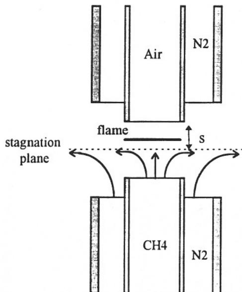
Figure 1. Schematic diagram of opposed-jet burner apparatus.
