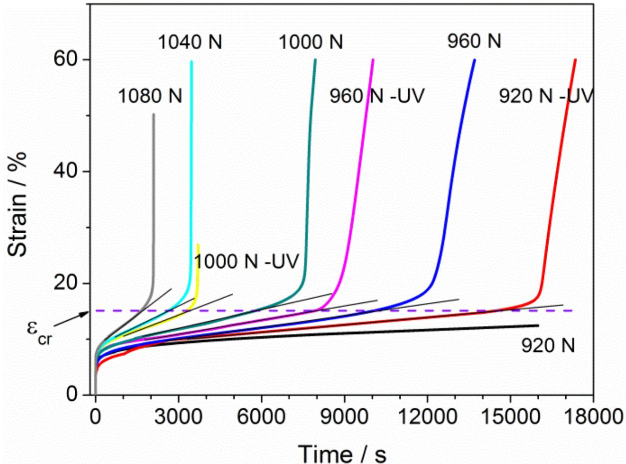
**The critical failure strain does not change with stress level and UV**
