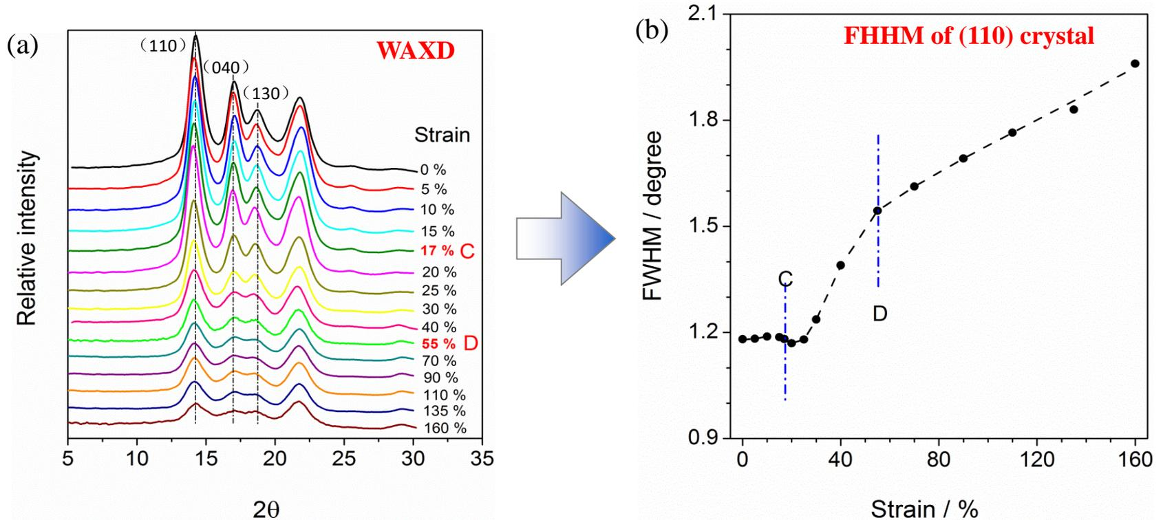
The FWHM of (110) crystal increased with strain, reflecting that the structural perfection of crystalline blocks in lamellae were reduced.
