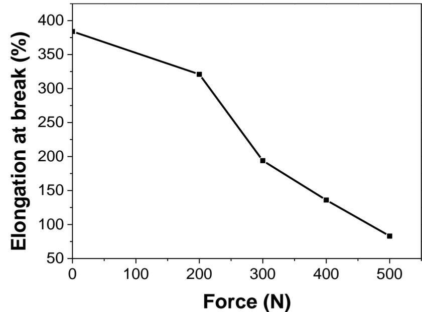
**Stress promoted chemical degradation and mechanical deterioration**
