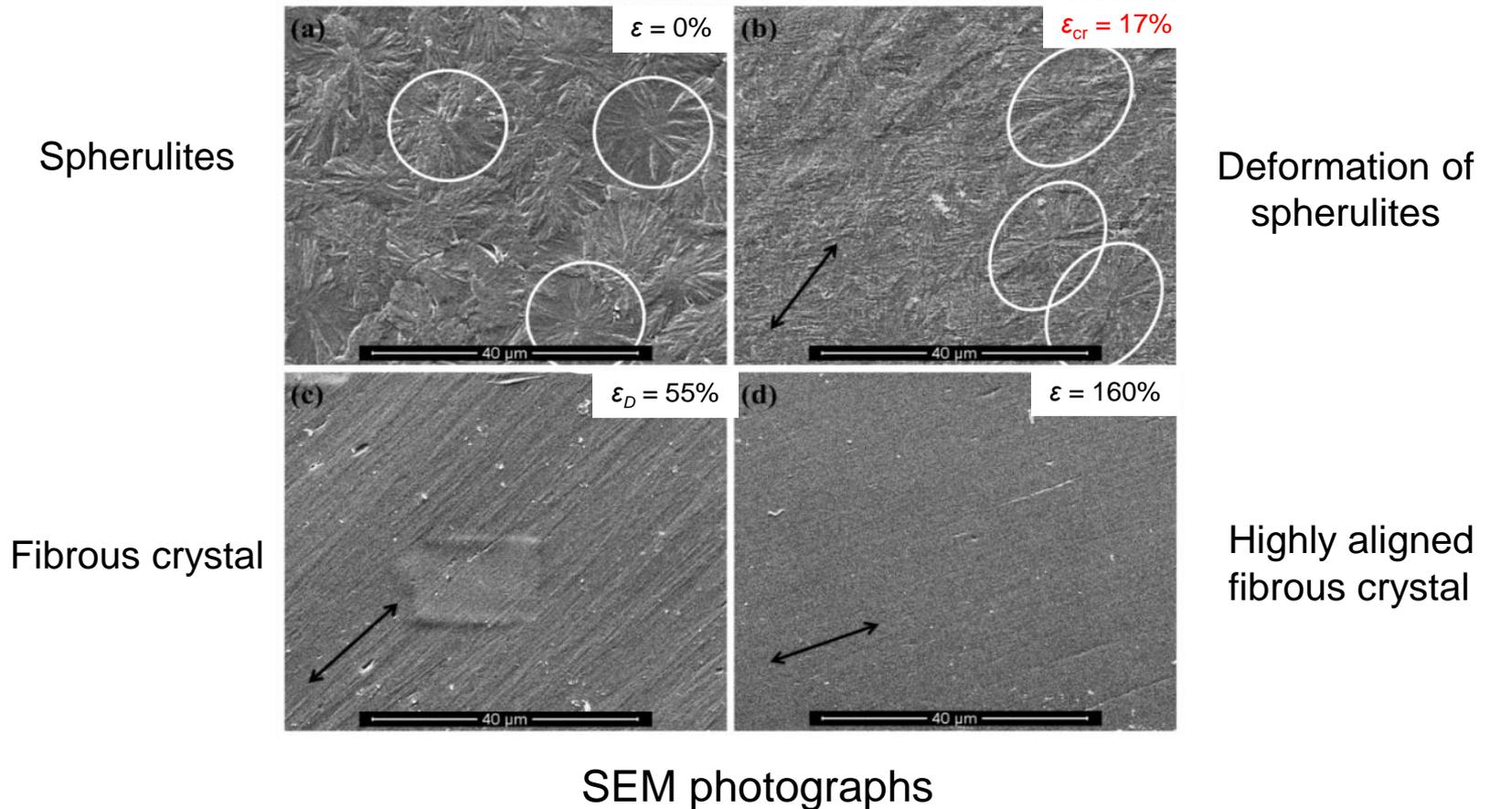
**The spherulites transformed into fibrous crystal with increasing strain**
