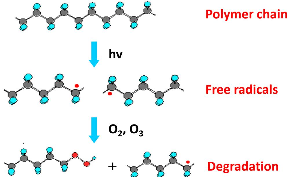
Failure or deterioration of materials due to the **degradation or crosslinking** of polymer chains in the presence of heat, oxygen, UV light, humidity, etc.
