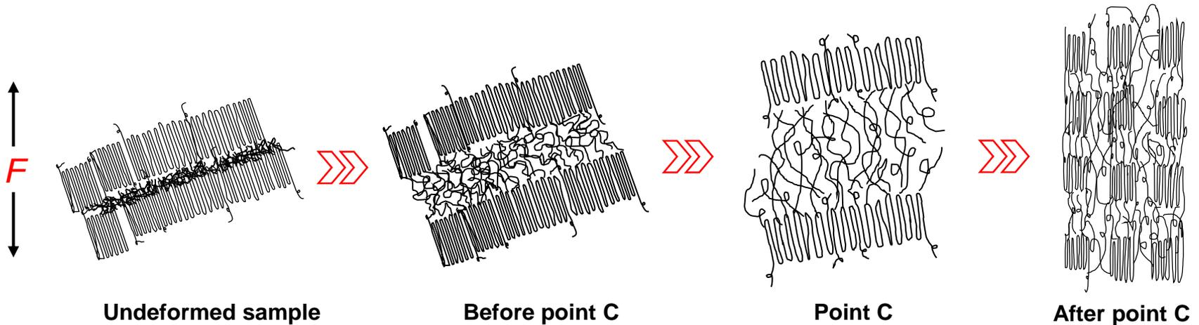
**Less deformation (before point C):** the entangled molecular chains in the amorphous region were stretched by the force (Long period  $d_{ac}$  rise)
