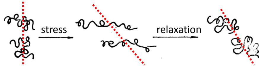
Failure or deterioration of polymers caused by the **creep or relaxation of polymer chains** in the presence of heat, stress, etc.
