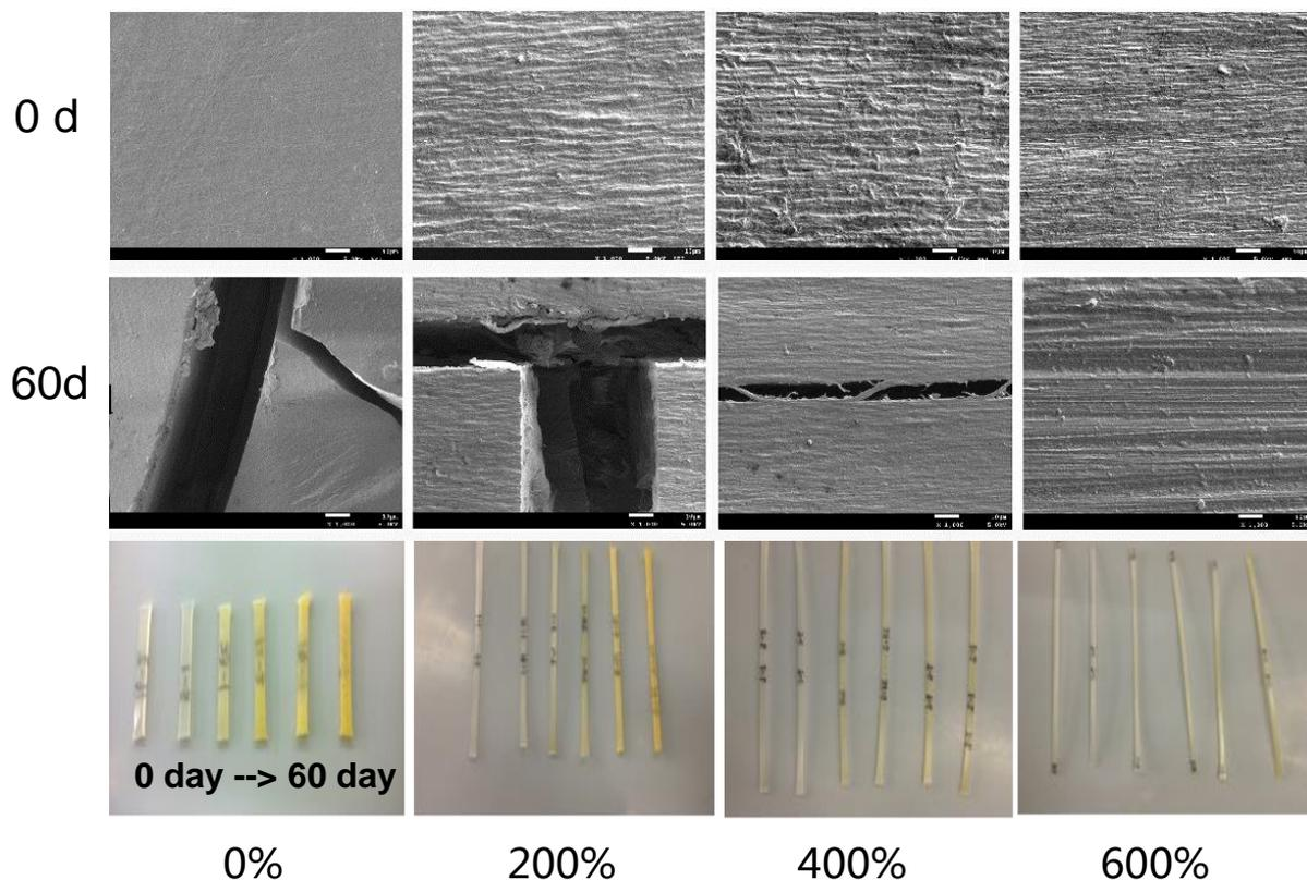
SEM and photographs of PA6 samples after been immersed in hot water (85°C) for 60 days
