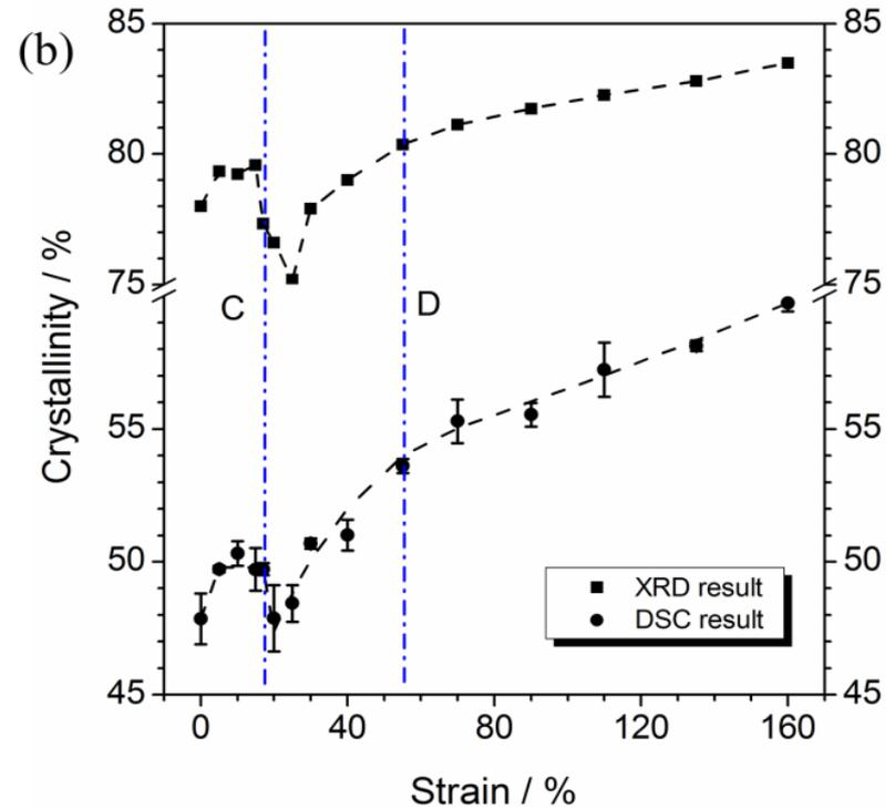
**The stress induced the process of crystalline block disaggregation-recrystallization.**
