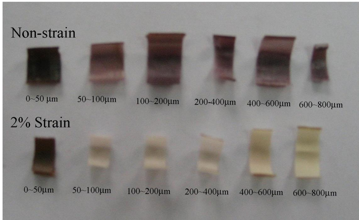
Color of sliced sample at different depths (irradiated for 20 days)
