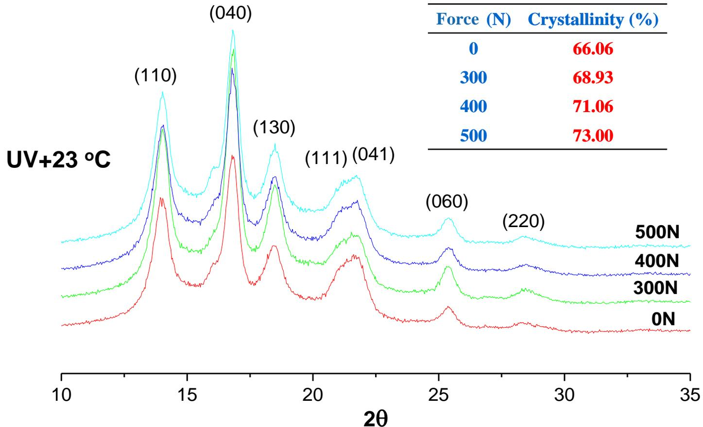
Higher stress increased the crystallinity and orientation, reducing the oxidation degradation (diffusion of oxygen) of iPP
