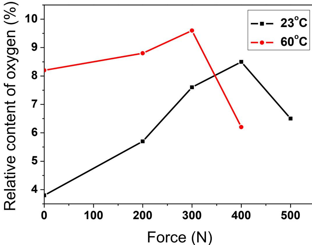
**With increasing stress level, the photo-oxidation degree increased at first and then decreases at higher stresses (XPS)**
