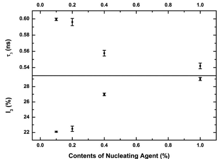
**The defects inside the material decreased with increasing content of nucleating agent, which are in favor of the improvement in creep resistance.**
