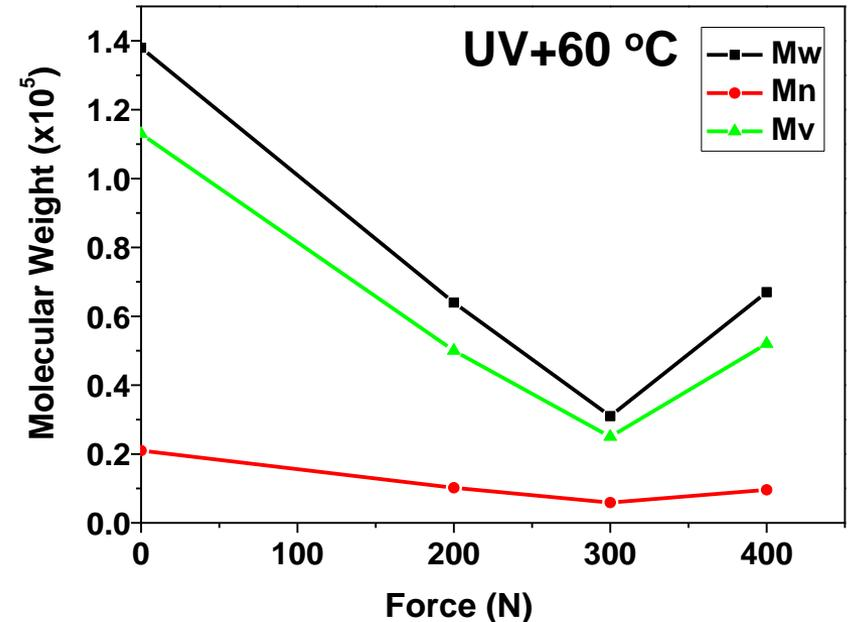
Molecular weight of iPP subjected to different stress levels after photo-oxidation for 12h
