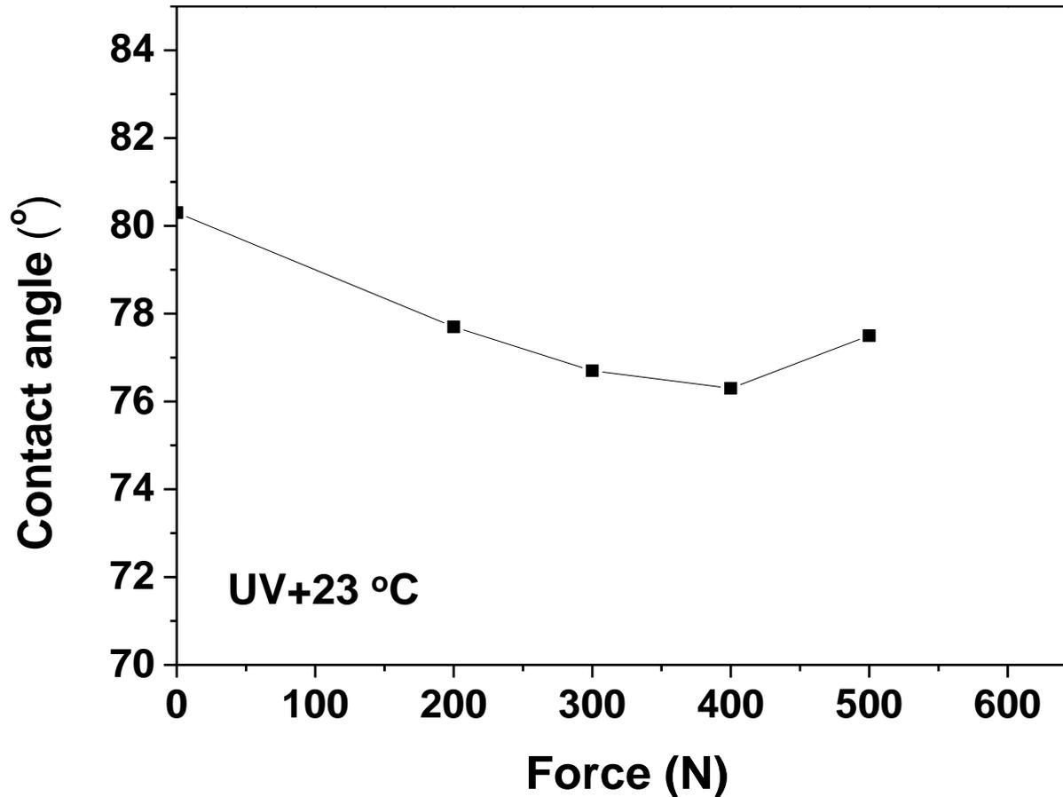
With increasing stress level, the contact angle decreased at first and then increases at higher stresses
