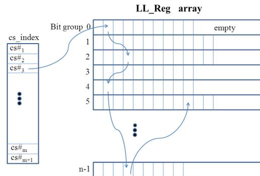
Figure 4. GPU Mini-Lookup data structure.
