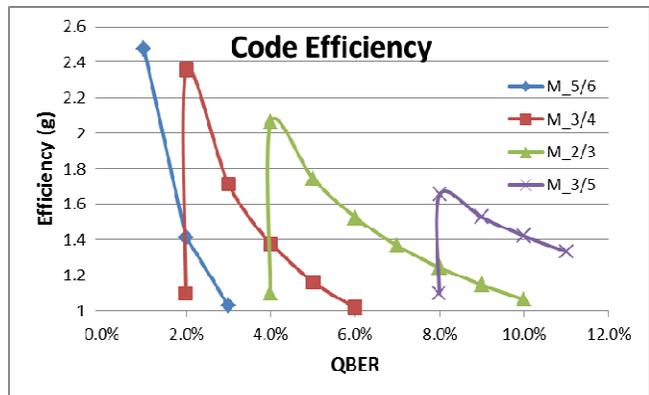
Figure 7. Error Correction Efficiencies for our LDPC Matrices.
