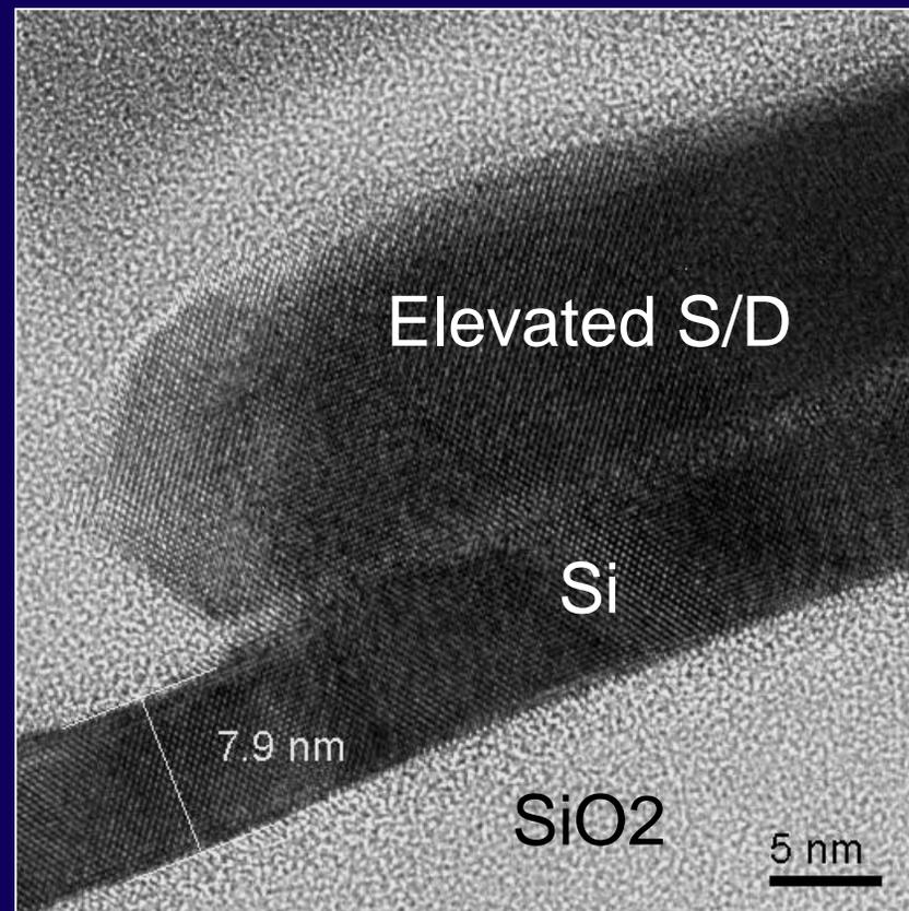
Excessive Silicon etching during surface cleaning steps may influence channel characteristics
