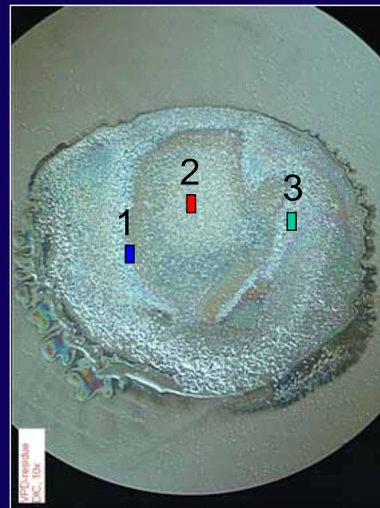
ToF-SIMS analysis (left) at different locations within the droplet (right) shows its constant chemical composition
