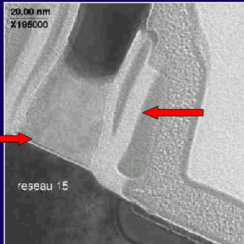
2-D spacer shape affects transistor characteristics !
