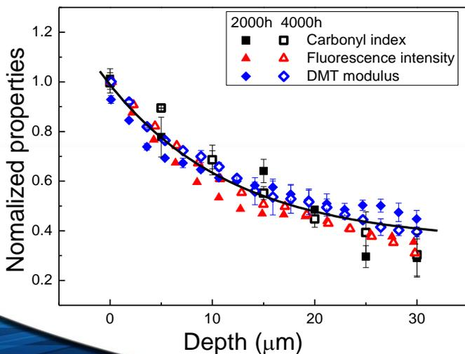
For the UV exposed side of the cross-sections,
