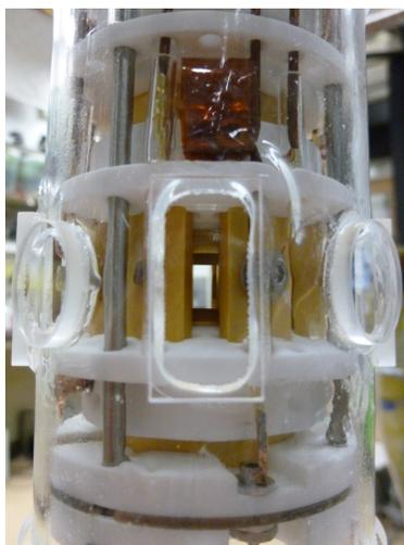
Figure 3.4: Photograph of trap inside fused silica vacuum envelope. The view is that of the ODF beam path through the trap.
