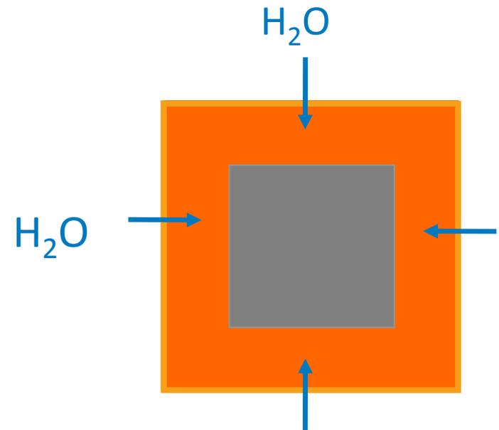
Ca test samples PIB #2 based, desiccant filled edge seal. Samples are 50 mm by 50 mm.
