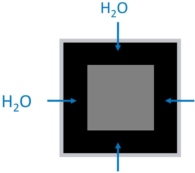
Moisture ingress measured at 45°C and 85°C, with RH held at 85%, and at lower levels using saturated salt solutions of LiCl, MgCl, or NaNO<sub>3</sub>.
