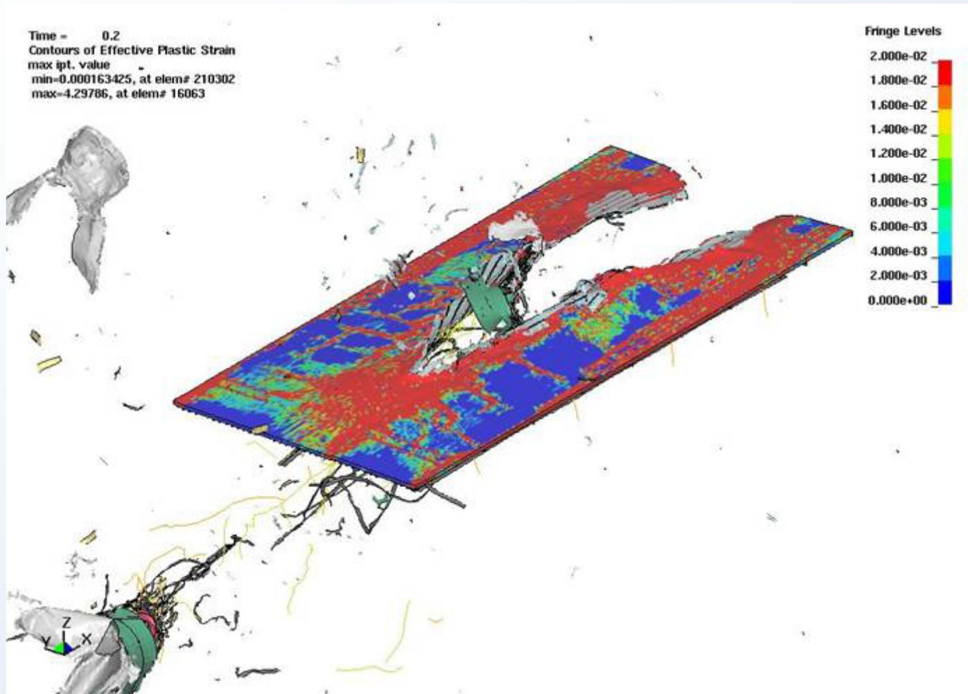
Fine Brick Element Floor Section Model
