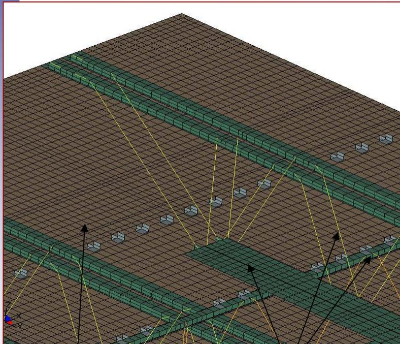
Smeared Concrete & Metal Decking Shell Model
