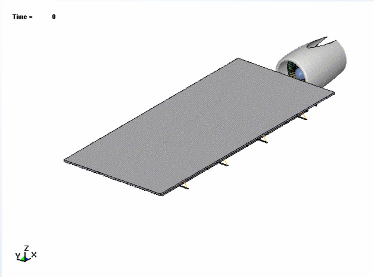
Fine Brick Element Floor Section Model
