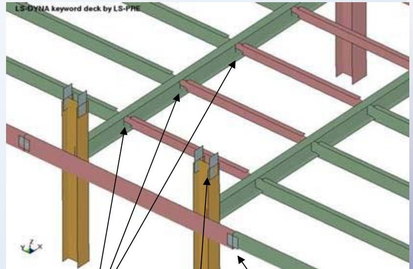
Node-to-Surface Tied Interface at Floor Beam Connections
