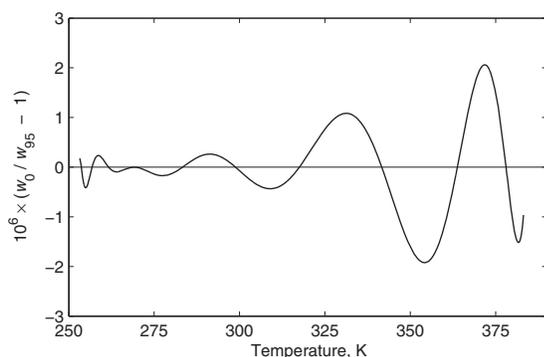
FIG. 3. Relative deviation of the speed of sound at 0.1 MPa given by the present formulation from the IAPWS-95 formulation.<sup>1,2</sup>
