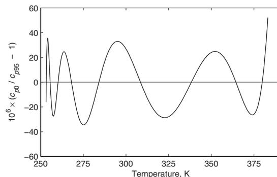
FIG. 2. Relative deviation of the specific isobaric heat capacity at 0.1 MPa given by the present formulation from the IAPWS-95 formulation.<sup>1,2</sup>
