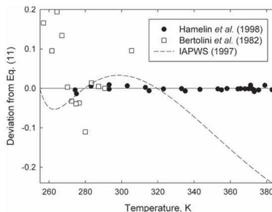
FIG. 7. Deviation of accepted dielectric-constant data from Eq. (11).
