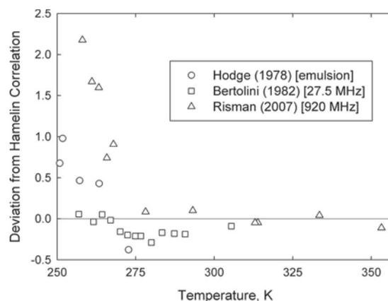
FIG. 6. Deviation from the correlation of Hamelin *et al.*<sup>18</sup> of dielectric-constant data from studies that measured data for supercooled water.
