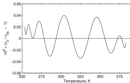
FIG. 1. Relative deviation of the specific volume at 0.1 MPa given by the present formulation from the IAPWS-95 formulation.<sup>1,2</sup>
