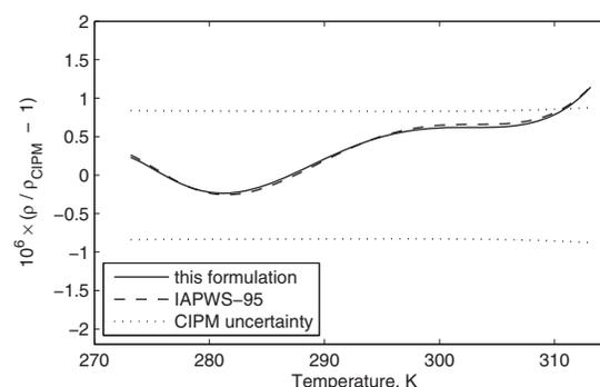
FIG. 4. Relative deviation of the density at 0.101 325 MPa given by the present formulation [reciprocal of  $v_{\text{atm}}$  from Eq. (6)] and by the IAPWS-95 formulation<sup>1,2</sup> from the CIPM recommended values for the density of water between 0 and 40 °C.<sup>15</sup>
