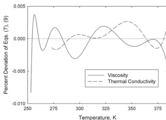
Fig. 5. Relative deviation of correlations for viscosity [Eq. (7)] and thermal conductivity [Eq. (9)] from the corresponding IAPWS standards.
