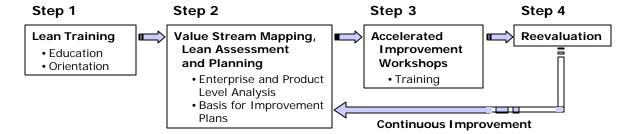
customer. Lean manufacturing differs from traditional manufacturing in that traditional manufacturing philosophies stress high utilization of machines and manpower with less emphasis on cycle time or manufacturing waste. Typical benefits from lean manufacturing include: productivity improvements, reduction in work-in progress, increase in space utilization, improved quality, and reduction in lead times.
