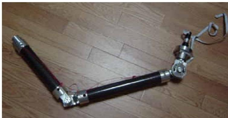
Figure -13 5 degree of freedom manipulator which has a multi-sensor head
