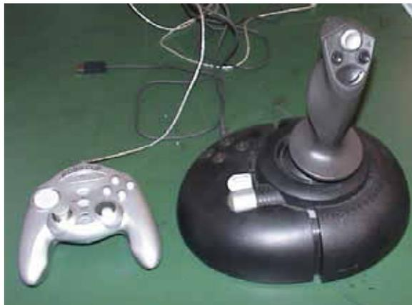
Figure -6 A joystick for the robot control and a joy pad for the manipulator control
