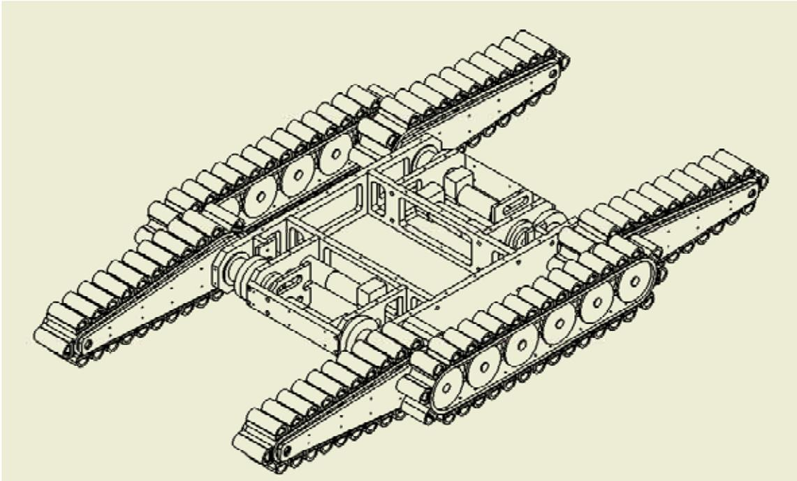
Figure -7 The internal structure of rescue robot
