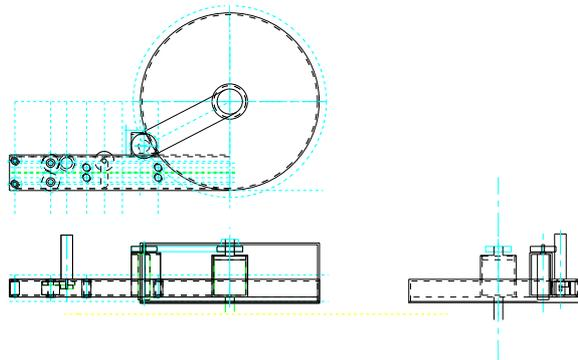
Figure -14 Wire wind device
