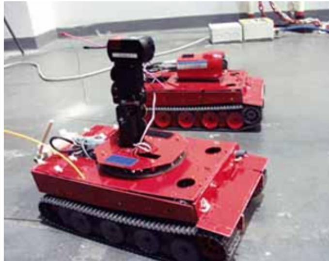
**Fig. 1.** MA1 & MA2 are small-size tank model robots that are driven independently, and have good mobility in flat surface environment.
