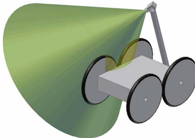
**Fig. 3.** FUMA is a middle-size four wheeled robot. Each side of the wheels can be driven independently. The arm mounted on the robot contributes high mobility to step over rough terrains and provides a high position camera viewing point (the robot is still under construction).
