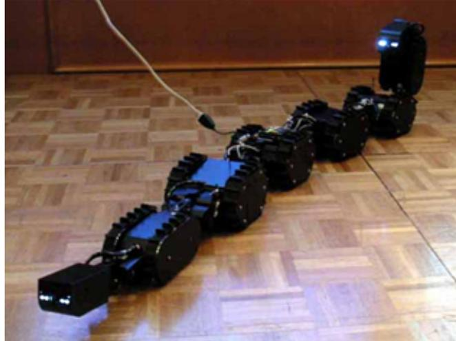
**Fig. 2.** KOHGA is a snake-type robot consists of eight units. Each unit has two tracks except the two heads. These units are serially interconnected with both ends first two joints as 2-DOF active joint and rest of the joints as 3-DOF passive joint. The passive joints provide good adaptation to complex environments. For this reason, KOHGA has high mobility even in rough terrains.
