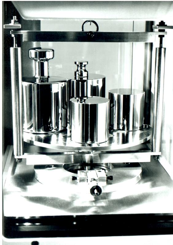
**Fig. 2.** The national standard of mass K20, K4, and secondary stainless steel standards inside the balance during measurement.
