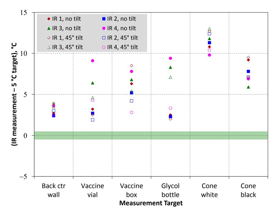
Figure 4. IR thermometers tested with targets in a large pharmaceutical refrigerator at 5 °C. The green zone represents an acceptable measurement range of ±0.5 °C around the 5 °C measurement temperature.
