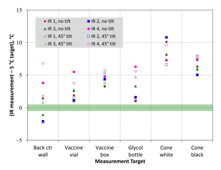
Figure 1. IR thermometers tested with targets in a dual-zone refrigerator at 5 °C. The green zone represents an acceptable measurement range of ±0.5 °C around the 5 °C measurement temperature.
