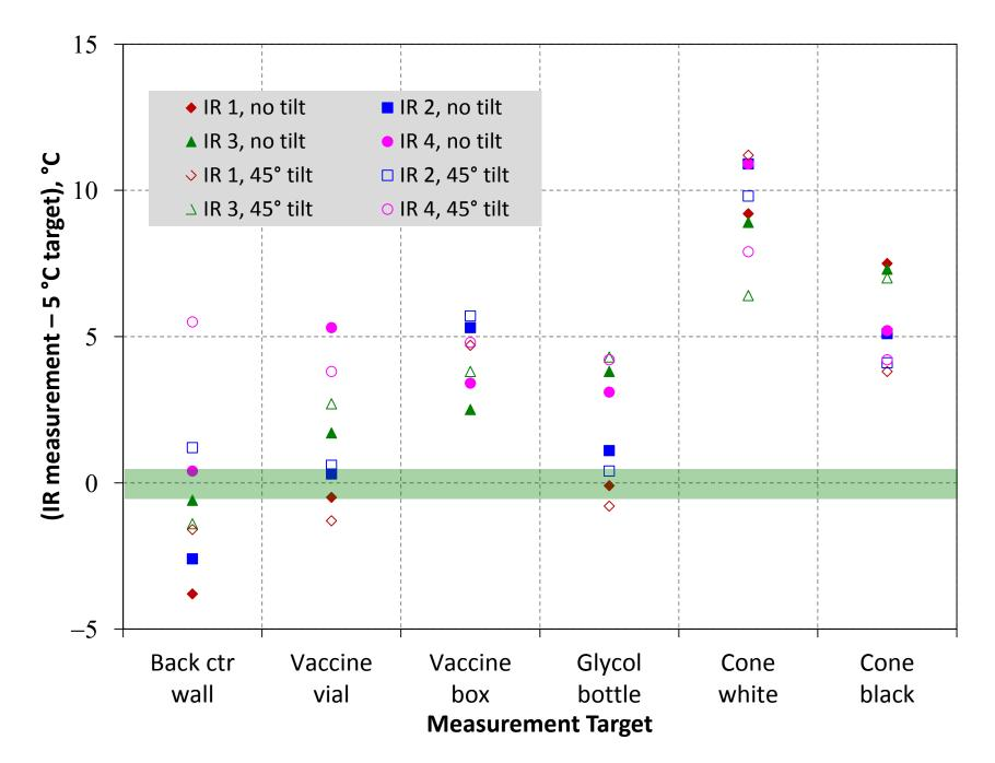
Figure 2. IR thermometers tested with targets in a freezerless refrigerator at 5 °C. The green zone represents an acceptable measurement range of ±0.5 °C around the 5 °C measurement temperature.
