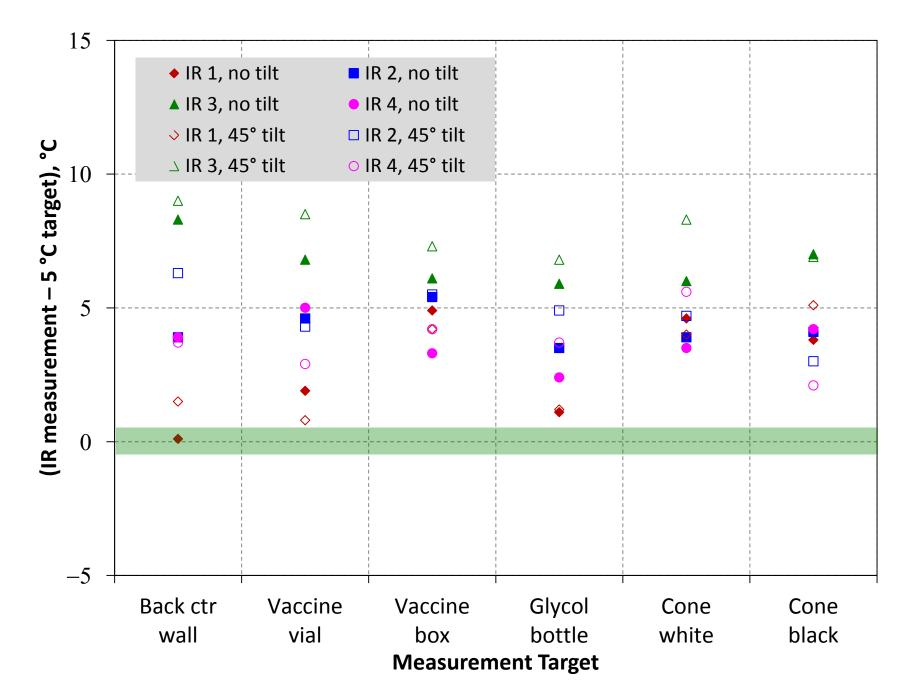
Figure 3. IR thermometers tested with targets in a small pharmaceutical refrigerator at 5 °C. The green zone represents an acceptable measurement range of ±0.5 °C around the 5 °C measurement temperature.
